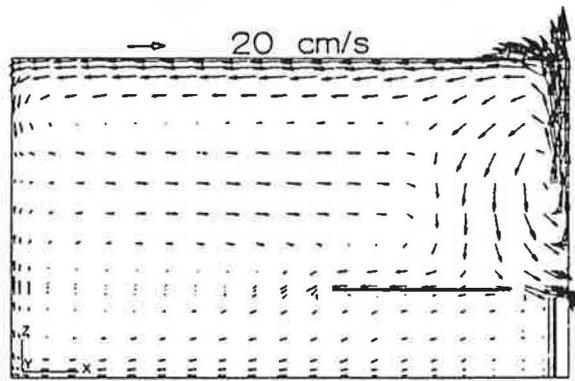
Figure 6 Airflow field of the room in section  $y/W=0.5$  computed by PHOENICS
