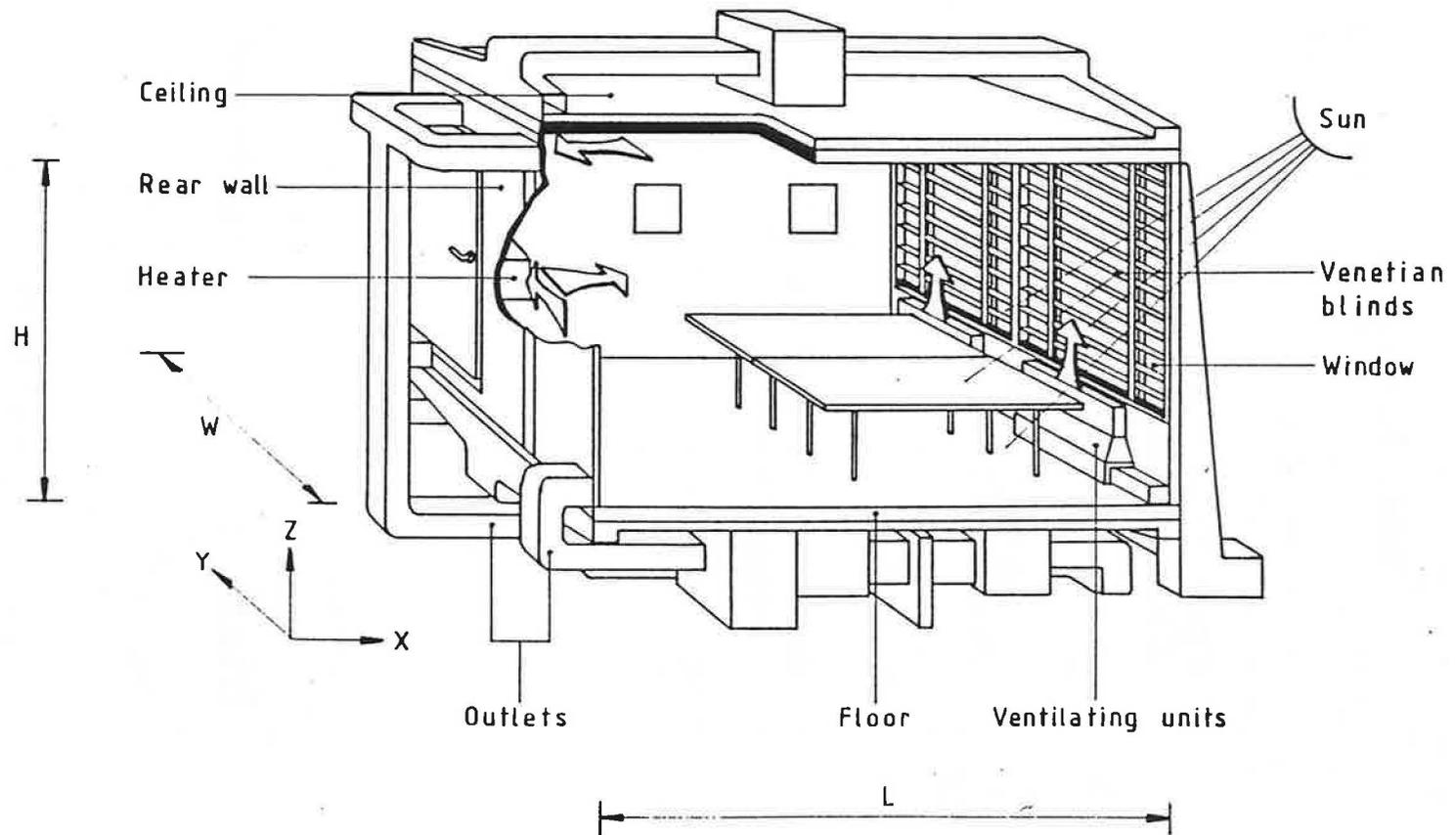
Figure 4 The climate room used for measurements
