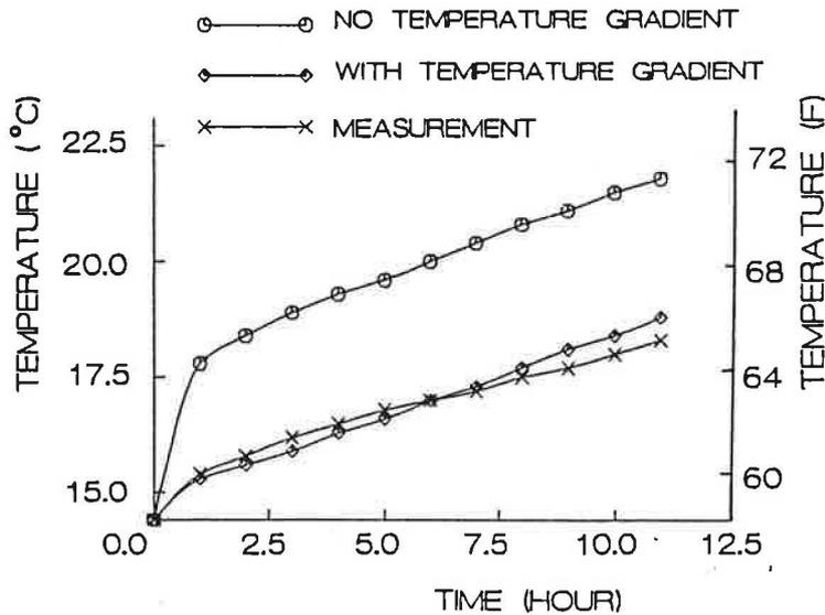
Figure 12 Computed and measured air temperature in the middle point of the room
