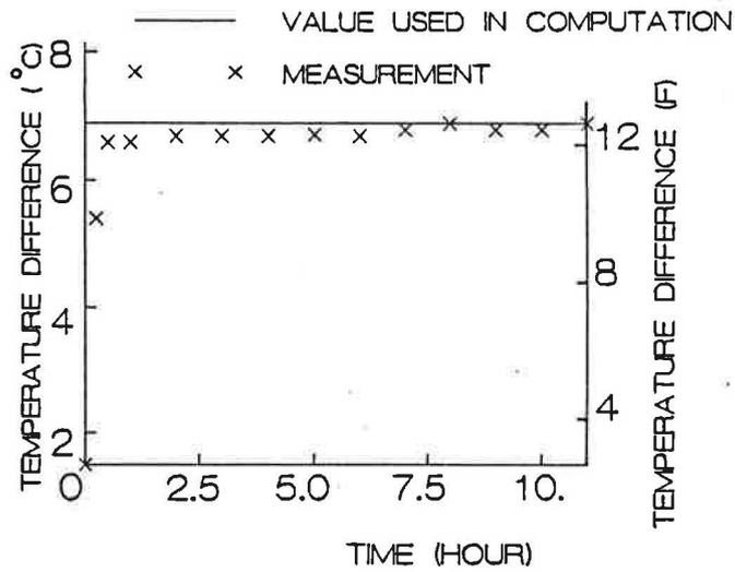
Figure 11 Temperature difference between the air points near the ceiling and the floor in the heating case
