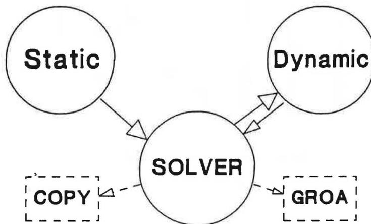
Figure 3 The structure for ACCURACY. COPY stores the numerical results as it appears in screen and GROA is the Graphical Representation Of Accuracy
