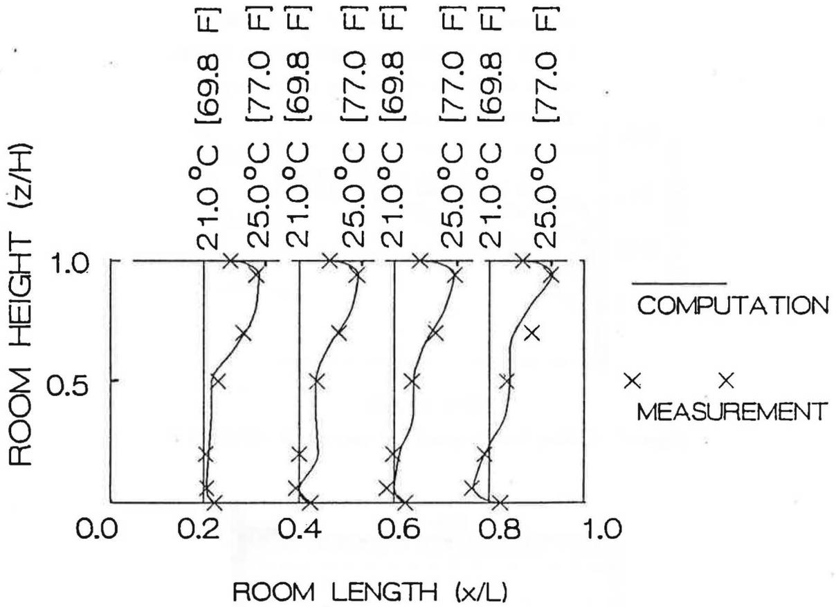
Figure 8 Temperature distribution of the room air in section  $y/W=0.5$
