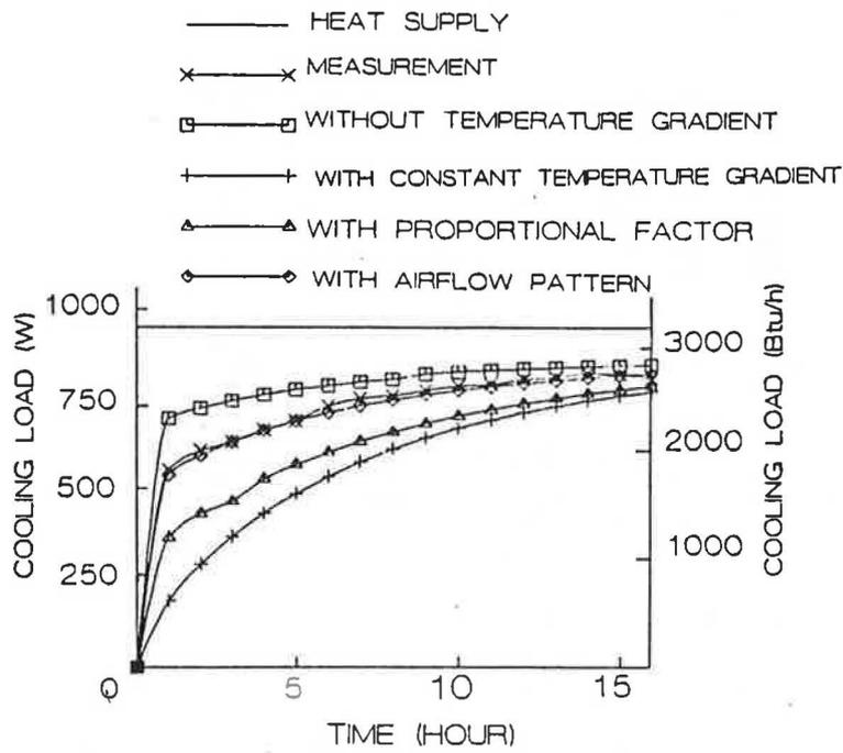
Figure 5 Cooling load measured and computed by ACCURACY
