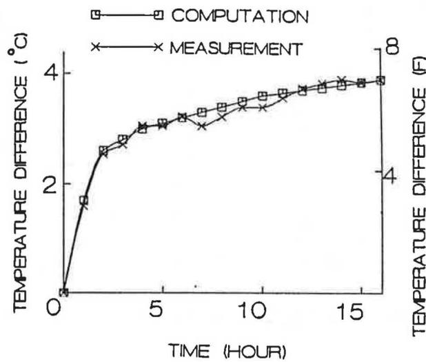
Figure 7 Temperature difference between the air points near the ceiling and the floor in the cooling case
