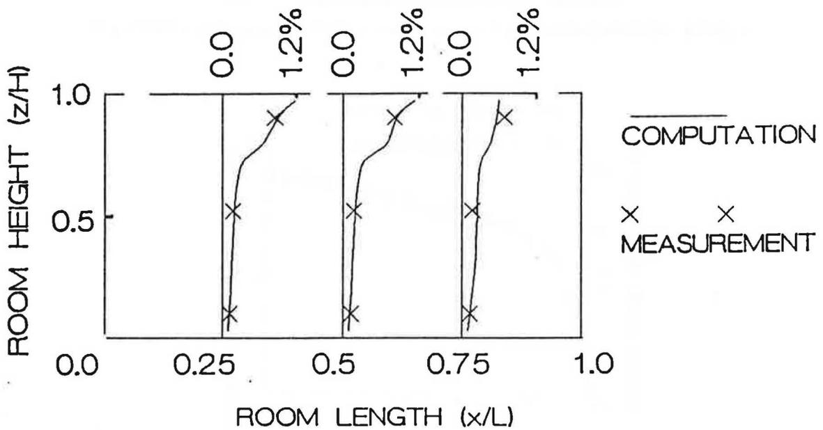
Figure 9 Contamination distribution of the room air in section  $y/W=0.5$
