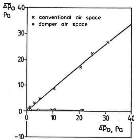
Figure 3.1.a. Mean pressure difference between air spaces over wall corner ( $\overline{\Delta P}_a$ ) as a function of mean pressure difference between outer surface of windward and leeward walls ( $\overline{\Delta P}_o$ ).
