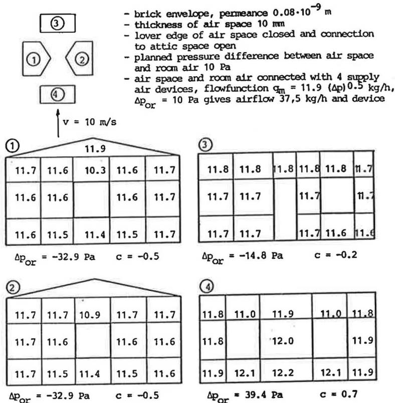
Figure 3.1.c. Computed pressure distribution in a damper air space of a  $10 \times 10 \times 2,5$  m<sup>3</sup> small house wall structure.  $\Delta p_{or}$  is pressure difference between outer surface and room air.
