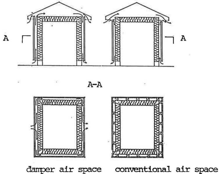
Figure 2.a. Principle of damper air space.
