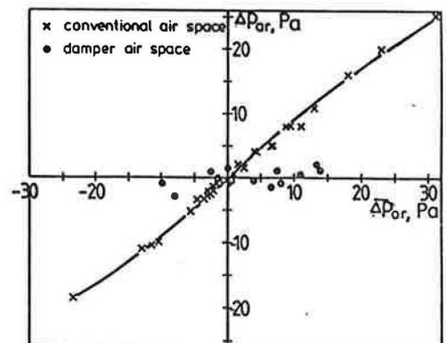
Figure 3.1.b. Mean pressure difference between air spaces and room air ( $\overline{\Delta P}_{ar}$ ) as a function of mean pressure difference between outer wall surface and room air ( $\overline{\Delta P}_{or}$ ).
