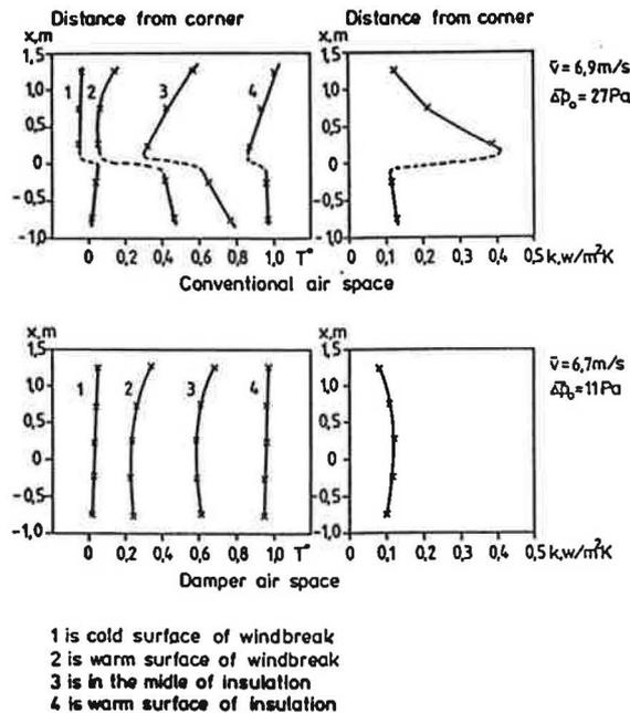
Figure 3.3.a. Horizontal distributions of relative temperature  $T^*$  at different depths in the wall structure and apparent k-value at the height of 1,25 m.
