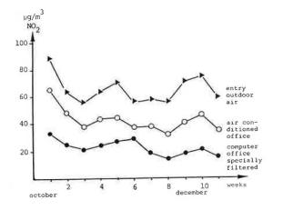
Fig. 1: Relation outdoor - indoor air in an air conditioned building in the town center.
