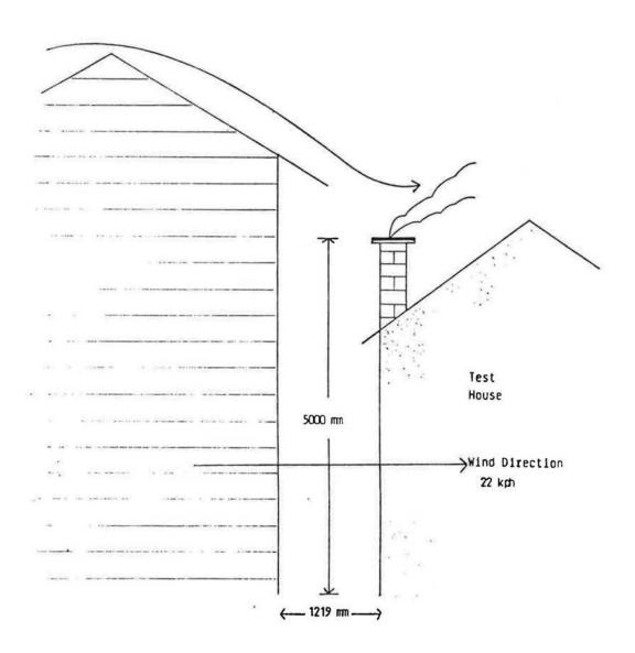
FIGURE 1: Geometry of Fireplace Chimney Clearance
