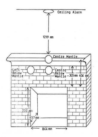
FIGURE 2: Location of Alarms and Dimensions of Test Fireplace
