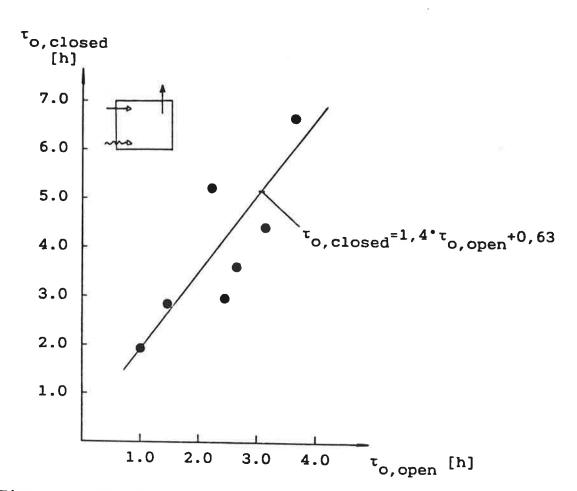
Figure 1. The impact of closing a door in dwellings on the airexchange rate. Natural ventilation./1/
