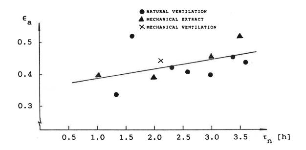
Figure 3. The air-exchange efficiency  $\varepsilon_a$  as a function of the nominal time constant  $\tau_n./1/$
