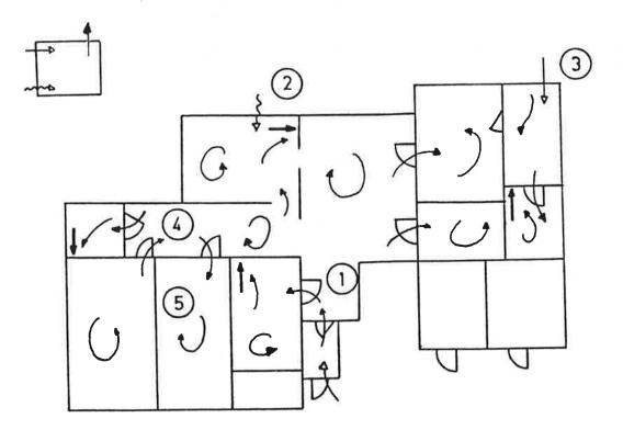
Figure 4. A typical air flow pattern in a dwelling./1/
