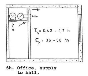
Figures 6c-h. Results of measurements with various ventilation patterns./2/
