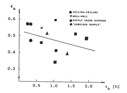
Figure 5. The air-exchange efficiency  $\epsilon_{a}$  as a function of a nominal time constant  $\tau_{n}$ . Office buildings./1/
