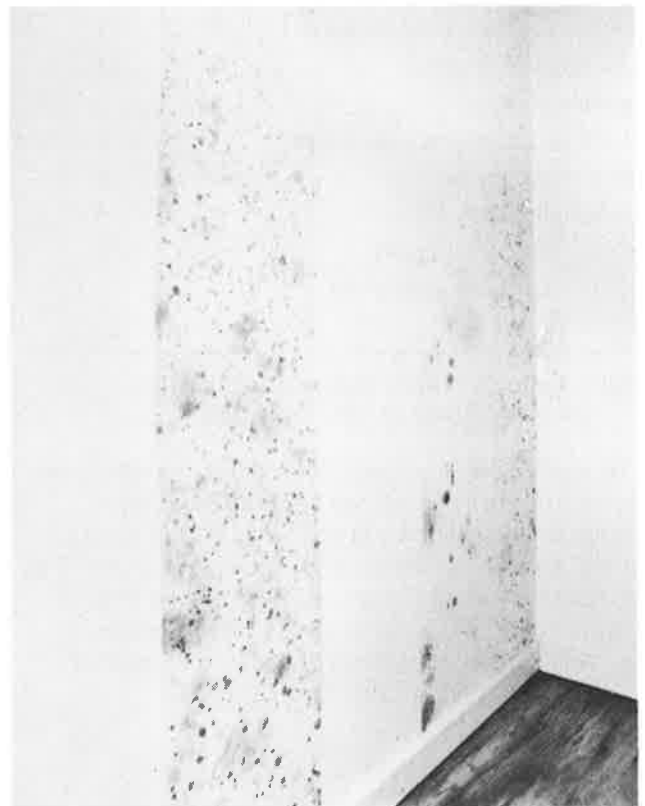
Figure 6 The test room at PRL clearly demonstrates the contrast between effective and non-effective fungicidal paints
