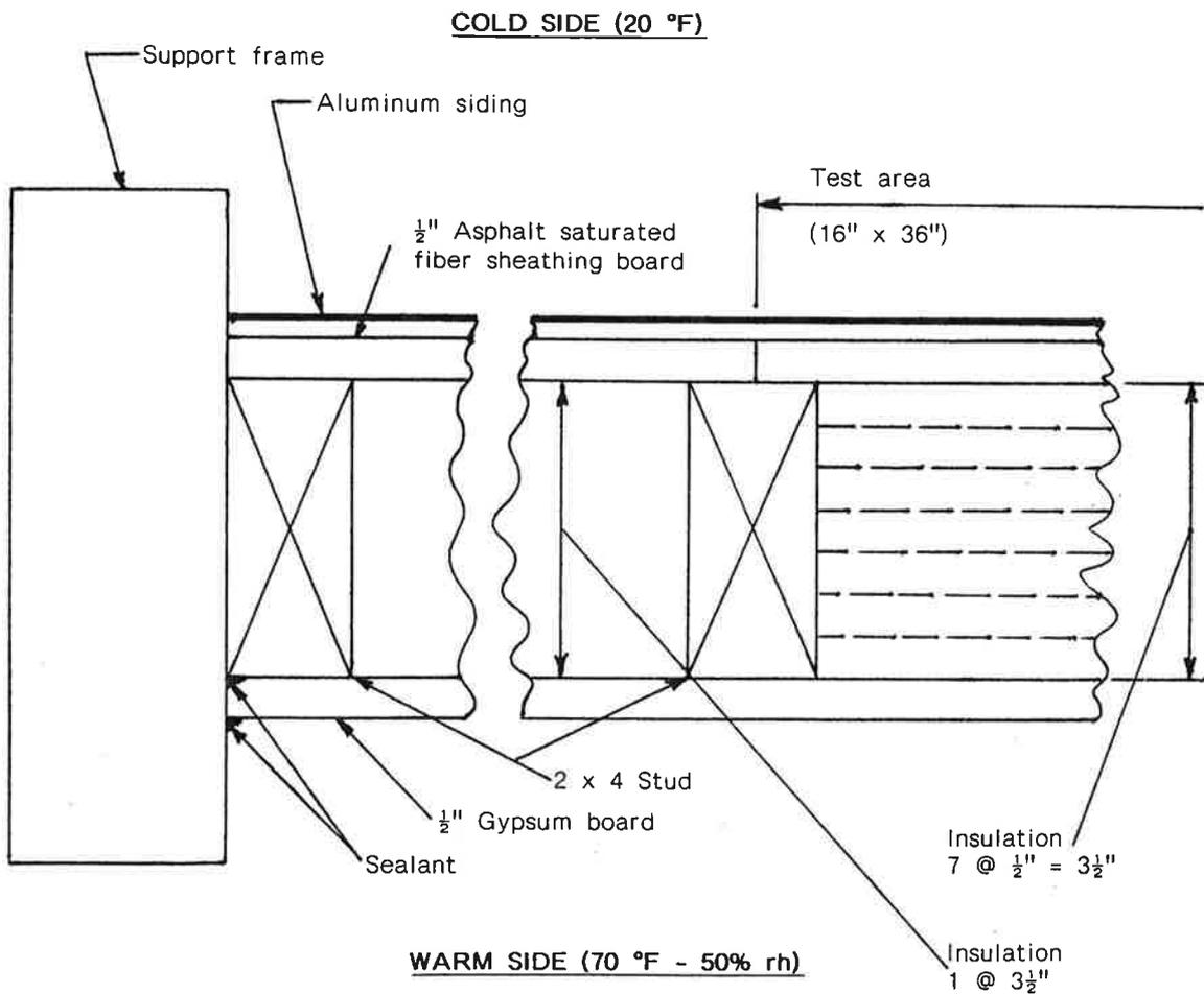
Figure 2. Moisture migration wall test panel - construction details
