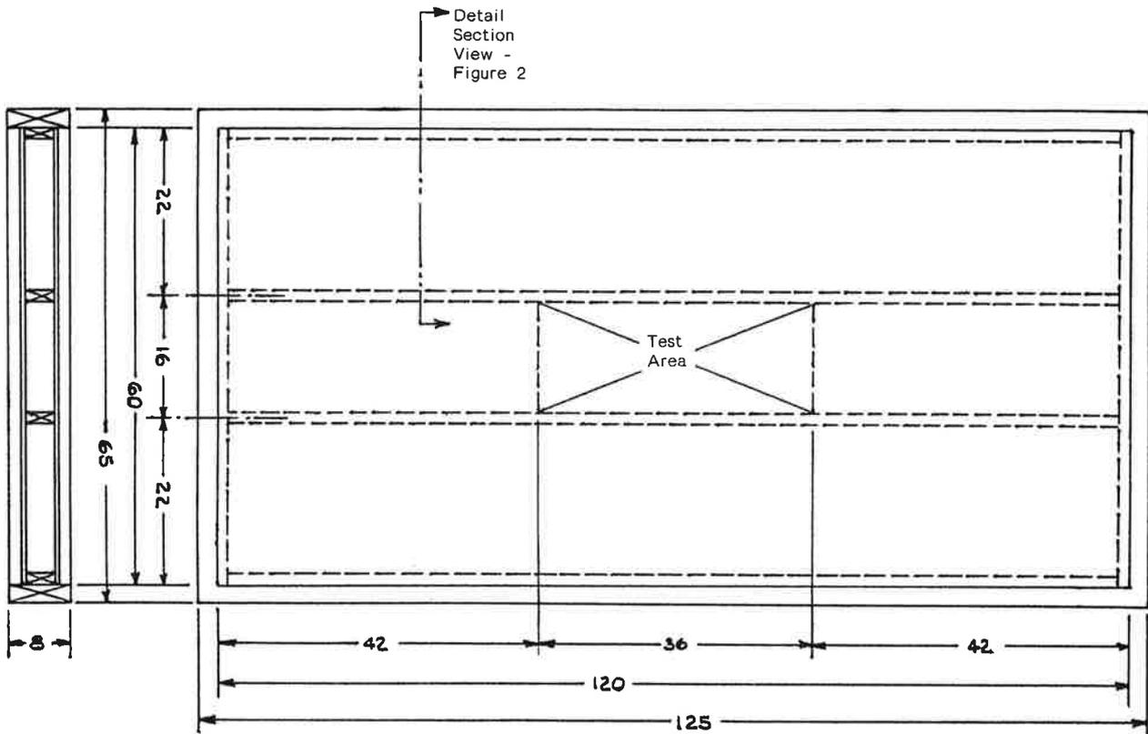
Figure 1. Moisture migration wall test panel
