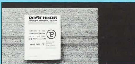
The U.S. Department of Housing and Urban Development has established standards for the amount of formaldehyde released from plywood and particle board to be used in mobile homes.
