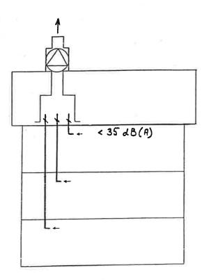
Fig.1 Simple mechanization of natural exhaust. Existing ducts are cut and provided with adjustable dampers. An exhaust fan is installed and the new ductwork is provided with noise reduction.
