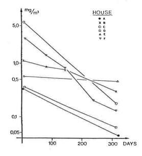
The change through 320 days of the total concentration of organic gases and vapours  $(mg/m^3)$  in six rooms.
