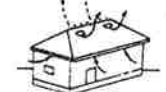
HIP ROOFS VENT AREA SHOULD BE EQUALLY DIVIDED BETWEEN EAVES & RIDGE WITH ALL VENTS SPACED EVENLY.
