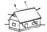
GABLE ROOFS HALF OF VENT AREA SHOULD BE IN THE GABLES OR AT A RIDGE VENT, WITH THE OTHER HALF AT THE CORNICE OR EAVES.
