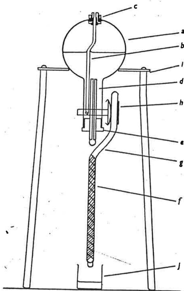
Fig. 2. Arrangements of dripping wick for acetone vapour determination. *a*, 100 c.c. round-bottom glass flask containing 0.2M hydroxylamine hydrochloride solution; *b*, air inlet tube of 3 mm. glass tubing; *c*, gland of stainless steel with rubber washer; *d*, capillary feed tube 6 cm. long, 0.5 mm. bore; *e*, rubber stopper; *f*, cotton bandage wound on; *g*, support of 5-6 mm. glass tubing; *h*, clip to support wick; *i*, stand, three-legged; *j*, 10 c.c. beaker.
