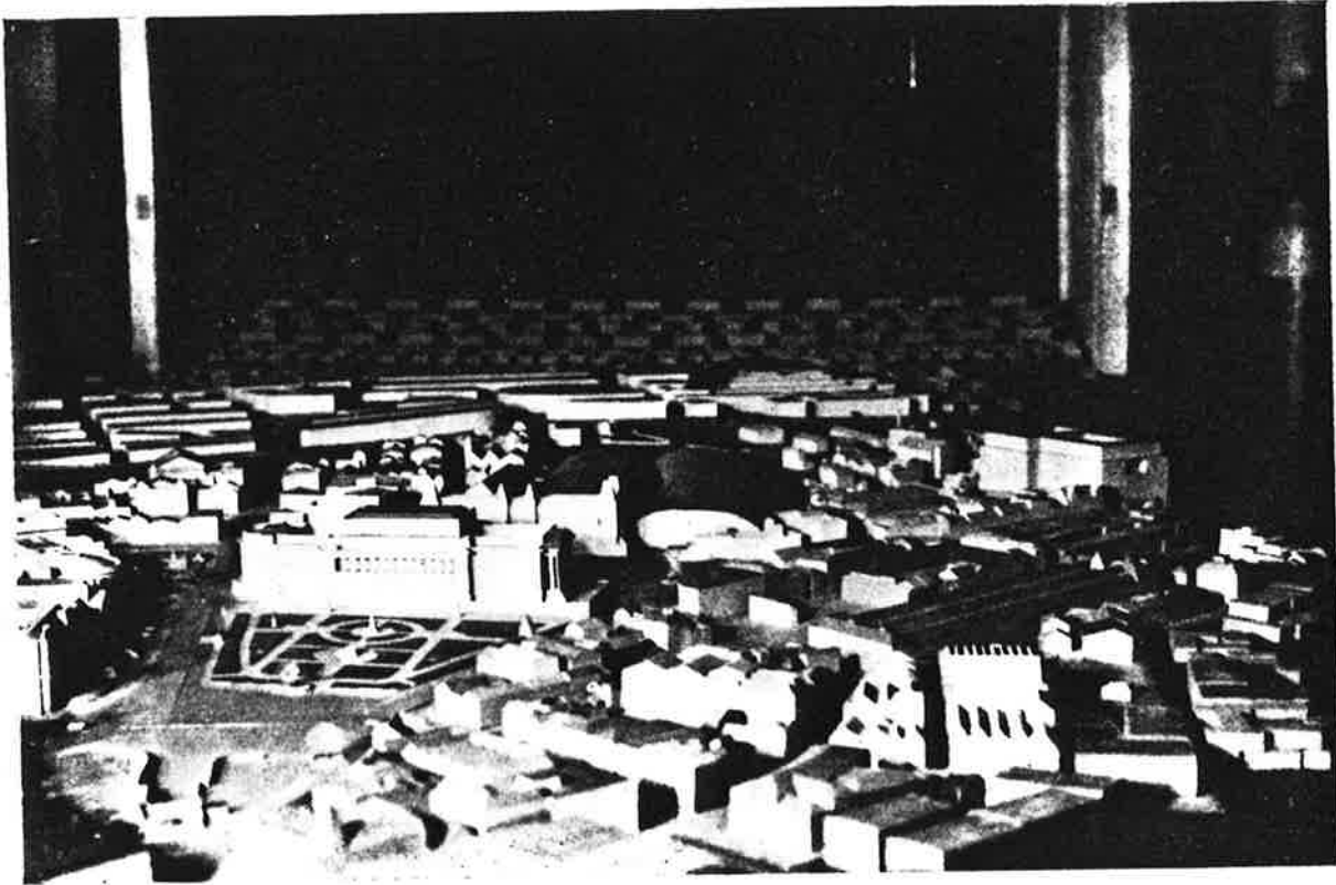
Fig. 4. Two views of the 1 : 500 scale model under test.
