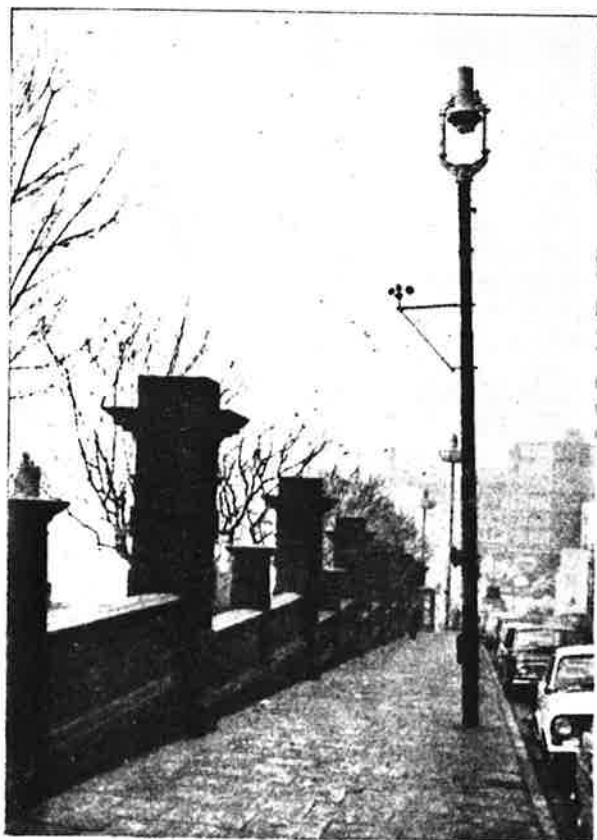
Fig. 3. Typical mounting of anemometer on lamp-post.
