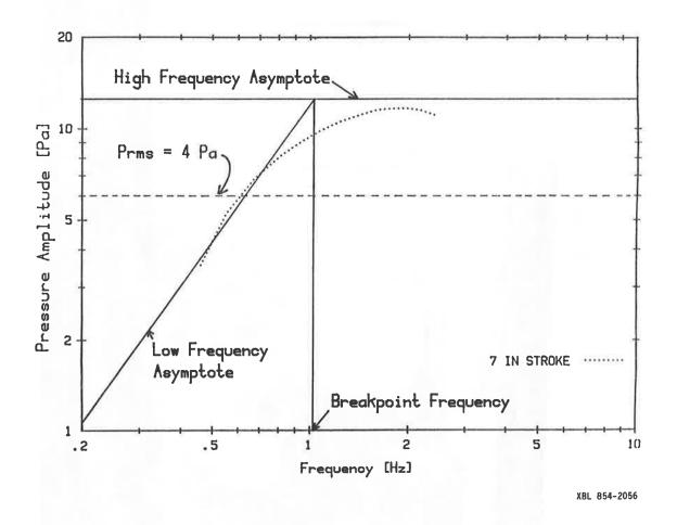
Figure 4. Sample pressure response versus frequency curve (house F).
