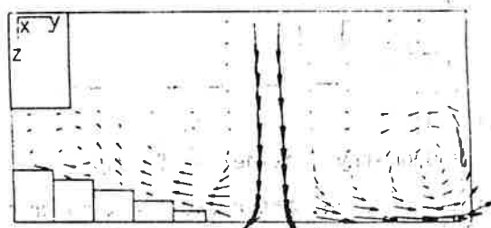
Fig. 3 Velocity vectors on the z-y plane passing through the middle of Studio 1 (max. velocity = 1.45 m/s)
