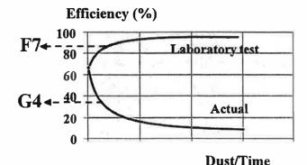
The classification is based on average efficiency during laboratory test. A filter tested to be a F7 filter in laboratory could be an G4 filter in an actual installation.
