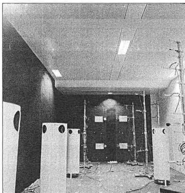
To test the Burgess chilled ceiling in a representative environment, a full-scale mock-up was built, measuring 7.2 by 3.4 m.
