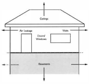
Heat loss is dependent on existing insulation levels and air tightness
