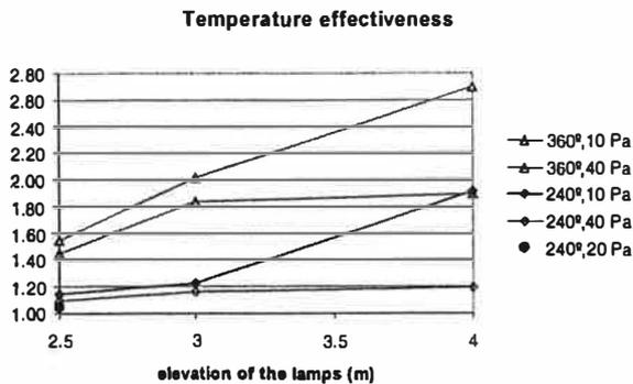
Figure 3. The temperature effectiveness vs. elevation of lamps
