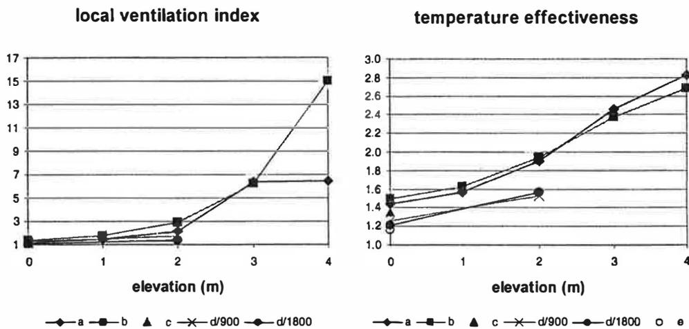
Figure 4. Measured temperature effectiveness and local ventilation index in the lower zone with convective heater.
