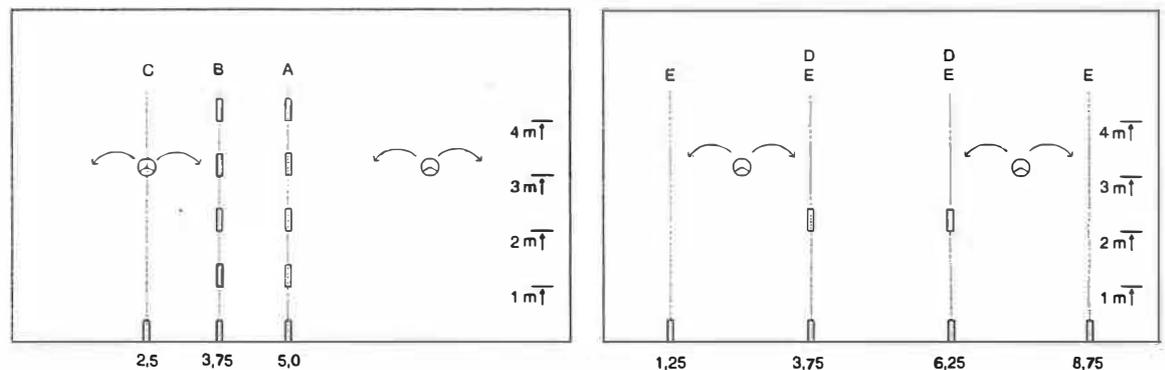
Figure 2a. The placement of the convector in test cases a, b and c (1 heater)
