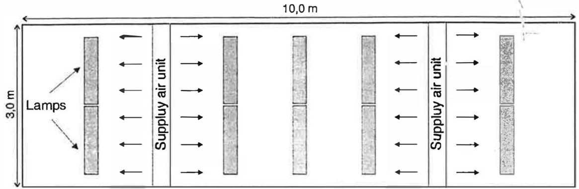
Figure 1. Plan view of the placement of the lamps
