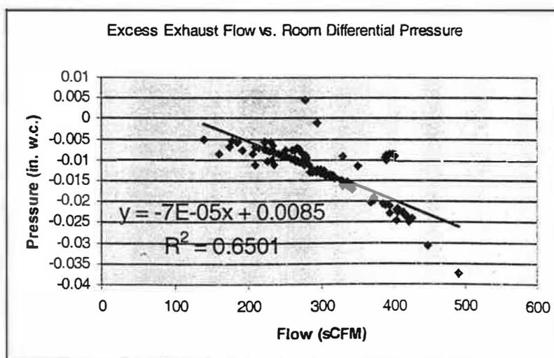
the patient room door resulted in a loss of established differential pressure, even with substantial excess exhaust. In Hospital C, the two rooms have a shared ante-room. The doors have sweeps on the bottom to prevent air from flowing readily into the rooms. The supply and exhaust rates in the room are nearly balanced resulting in slight negative pressure
