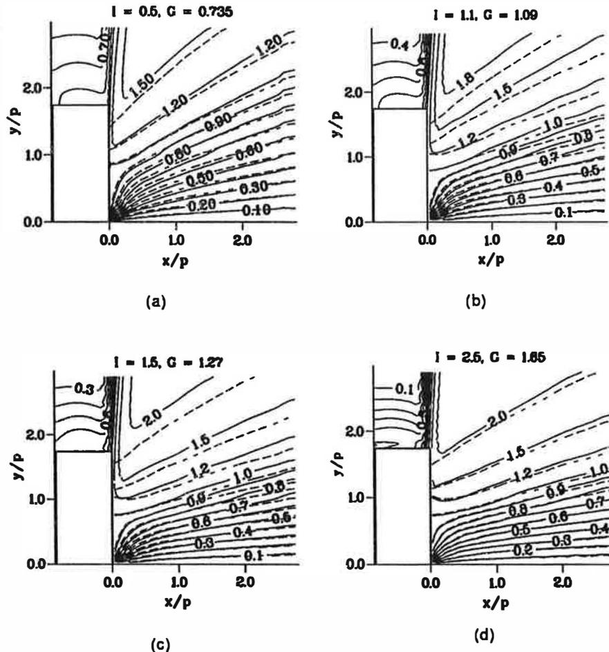
Figure 2. Streamlines when  $I = 0.5, 1.1, 1.5$  and  $2.5$ ,  $G = 0.735, 1.09, 1.27$  and  $1.65$ , -----  $k-\epsilon$  model, - - - potential model.
