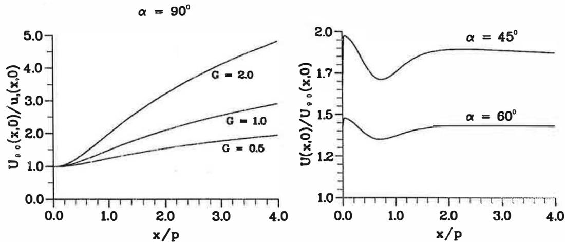
Figure 4. The ratio of velocities near to the surface of the workbench.
