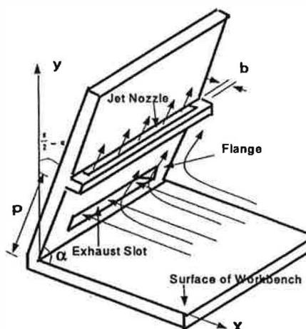
Figure 1. A schematic diagram of the Aaberg slot exhaust hood.
