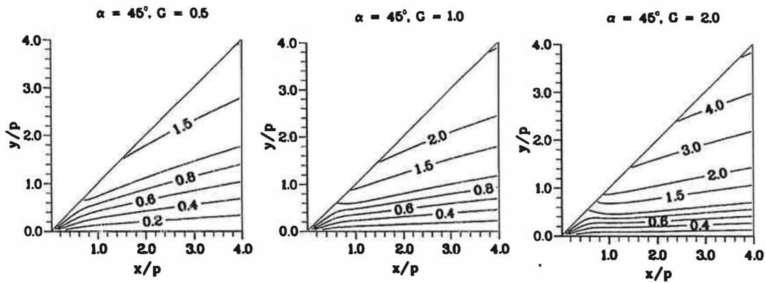
Figure 3. The streamlines of the air flow created by the Aaberg exhaust when  $\alpha = \pi/4$  and  $G = 0.5, 1.0$  and  $2.0$ .
