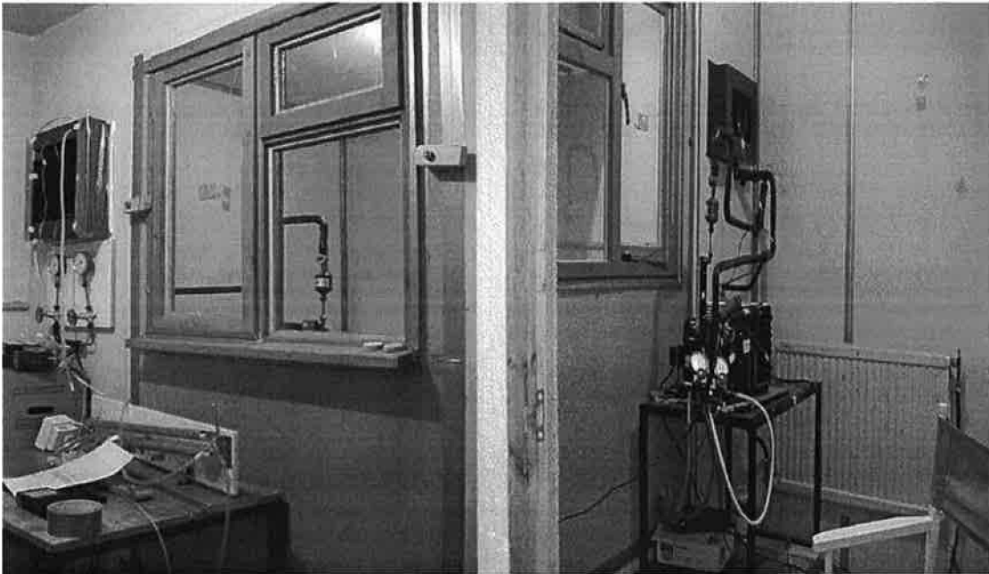
Fig: 4a. Indoor (left) and outdoor sides of the test chamber
