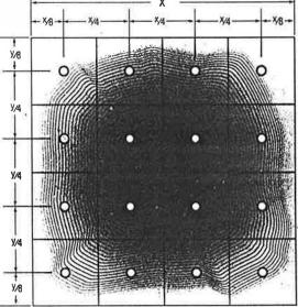
very good 107 percent of design outside-air flow directly to the space, but the main duct was traversed by the equal-area method to be 119 percent.
