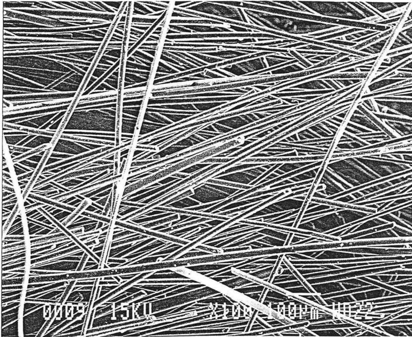
FIG. 12 SPECIMEN 2: VIRGIN CARBON FIBRE THREAD - END VIEW (X 100)
