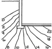
Soil temperatures in February under an insulated floor slab
