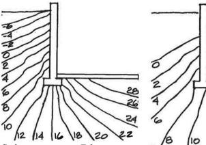
Soil temperatures in February under an uninsulated floor slab
