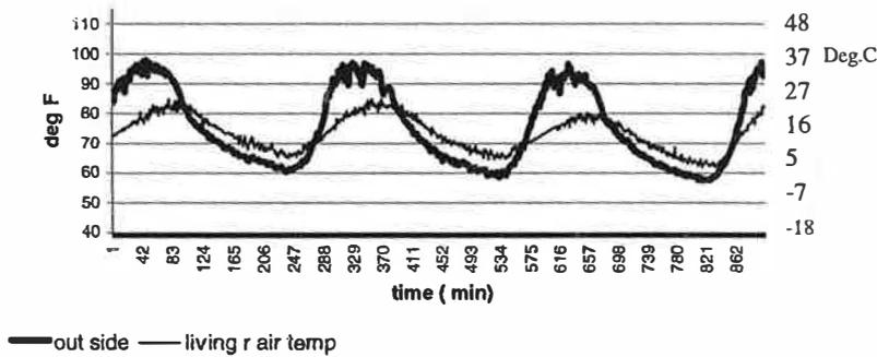
Figure 4: Passive house performance at hot periods with natural ventilation at night
