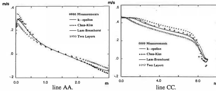
Figure 2 : Longitudinal velocity (in m/s), confrontation between experimental and numerical results for several turbulence models.
