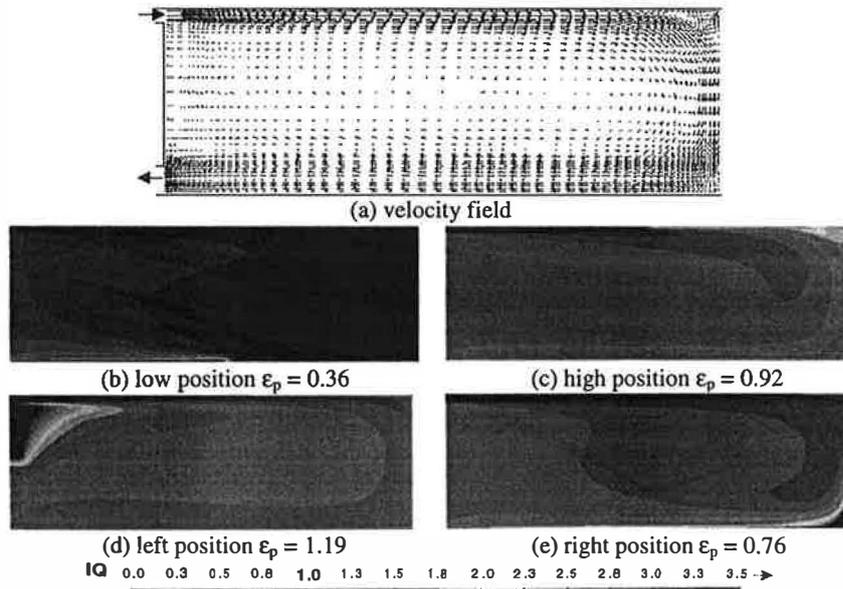
Figure 7 : Second configuration of exhaust, (a) velocity field, (b to e) IQ field for the different position of pollutant source.
