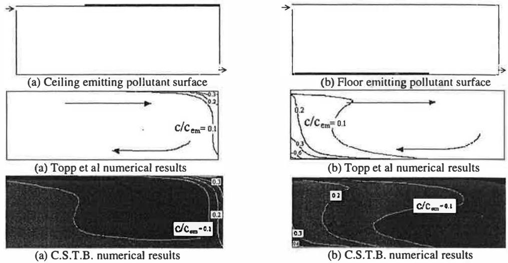
Figure 4 : Comparison of concentration distributions for two configurations (a) Ceiling emitting pollutant surface (b) Floor emitting pollutant surface.
