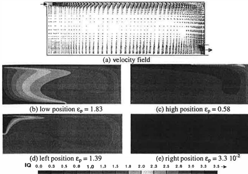
Figure 6 : First configuration of exhaust, (a) velocity field, (b to e) IQ field for the different position of pollutant source.
