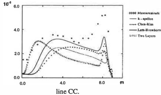
Figure 3 : Turbulence intensity, confrontation between experimental and numerical results for several turbulence models.
