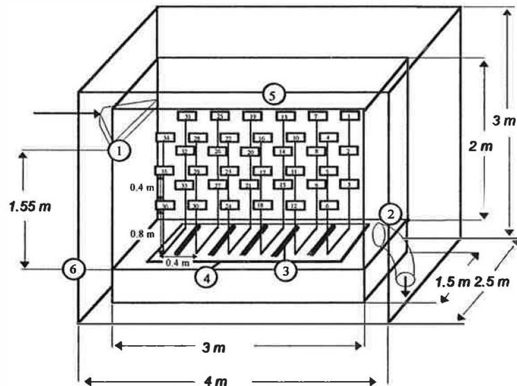
Figure 1: Schematic representation of the test room: 1. slotted air inlet; 2. air outlet; 3. heating element; 4. hot water reservoir; 5. grid of 36 thermocouples; 6. envelope chamber.
