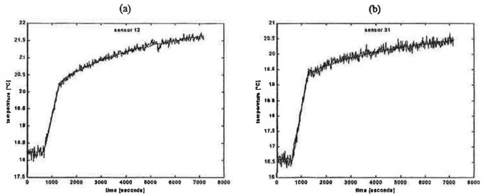
Figure 3: The output of the estimated model for sensor positions 12 (a) and 31 (b) in comparison with the measured temperature response data for an experiment with ventilation rate of 290 m<sup>3</sup>/h.
