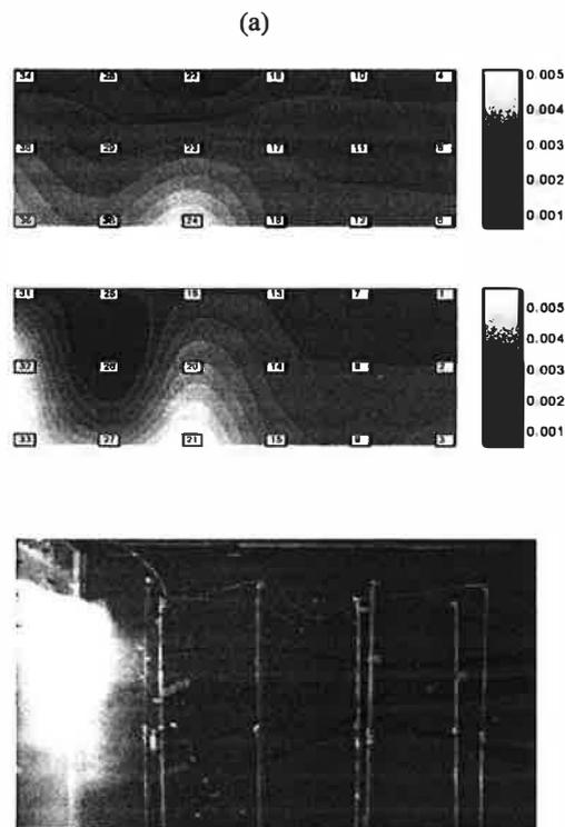
Figure 5: The spatial contours of the local outside air change rate in the front and rear sensor plane of the test chamber (a) and the visualised air flow pattern (b) at a low ventilation rate of  $150 \text{ m}^3/\text{h}$ .
