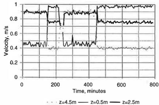
Figure 3. Velocities measured in the ceiling jet at the positions of  $x = 4.5 \text{ m}$ ;  $z = 0.5, 2.5, \text{ and } 4.5 \text{ m}$ ; and  $y = 2.98 \text{ m}$  (0.2m from ceiling) showing the semi-stable airflow statuses in the room.
