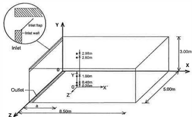
Figure 1. Room geometry and positions of inlet, outlet and sensors.  $a = 2.68\text{m}$ ,  $3.5\text{m}$  and  $4.5\text{m}$ .
