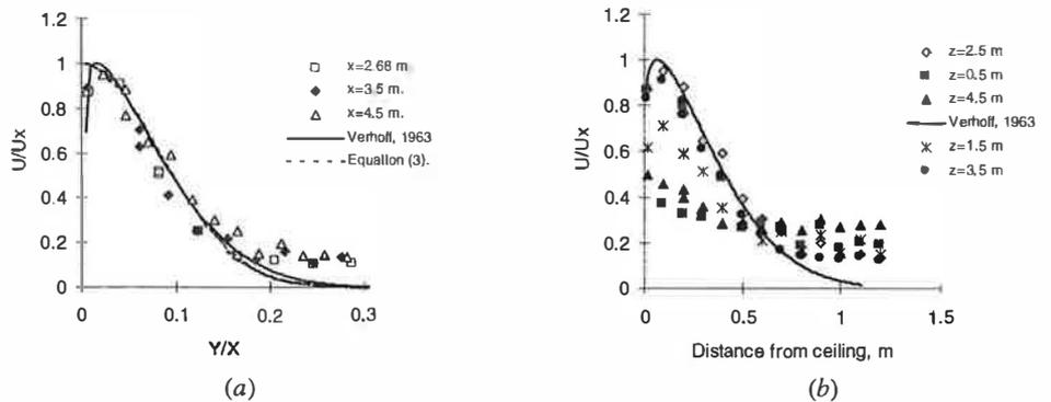
Figure 2. (a) Velocity profiles of the ceiling jet in the symmetric plane  $z = 2.5 \text{ m}$ . (b) Velocity profiles of the jet in five  $z$ -planes at the distance  $x = 4.5 \text{ m}$  from the inlet wall.
