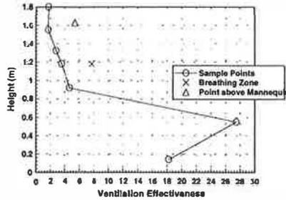
Figure 5: Ventilation effectiveness for DV1 configuration 2 with a seated mannequin
