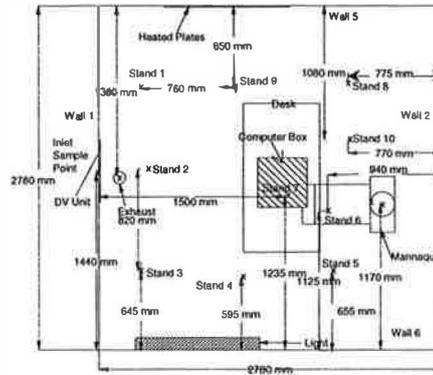
Figure 1: A plan of test compartment of the Reading Chamber and its contents
