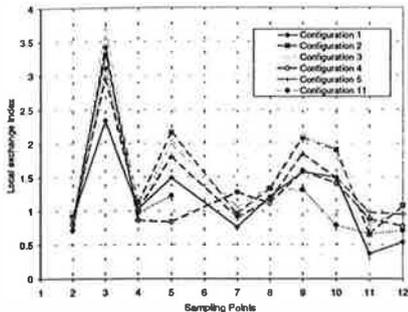
Figure 4: Local air exchange index for a seated mannequin for DV1
