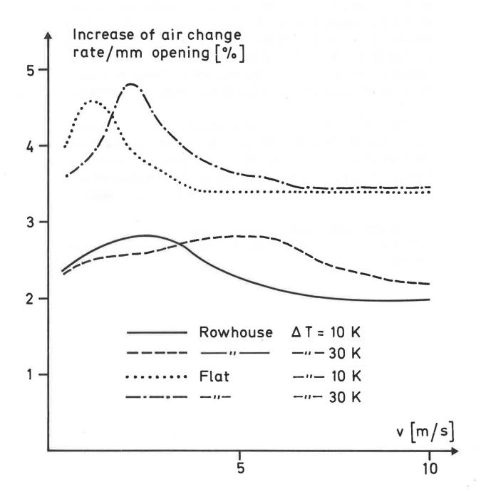
Fig 4 Increase in % of the rate of air change per mm effective opening width of the window, compared to the rate of air change when there are no open windows, versus the wind speed.
