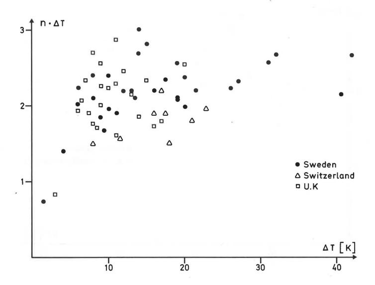
Fig 3 Fraction of rooms having open windows, n, times the indoor-outdoor temperature difference ΔT, versus ΔT. Data from eight studies (ref 4, 6, 7, 11 and this investigation) in Sweden, Switzerland and the UK.
