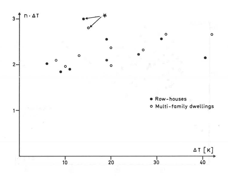
Fig 2 Fraction of rooms having open windows, n, times the indoor-outdoor temperature difference ΔT, versus ΔT. Data from observations of row-houses and multi-family buildings performed in this investigation. Data points indicated by an asterisk refer to days when there was someone at home in a large fraction of the households.
