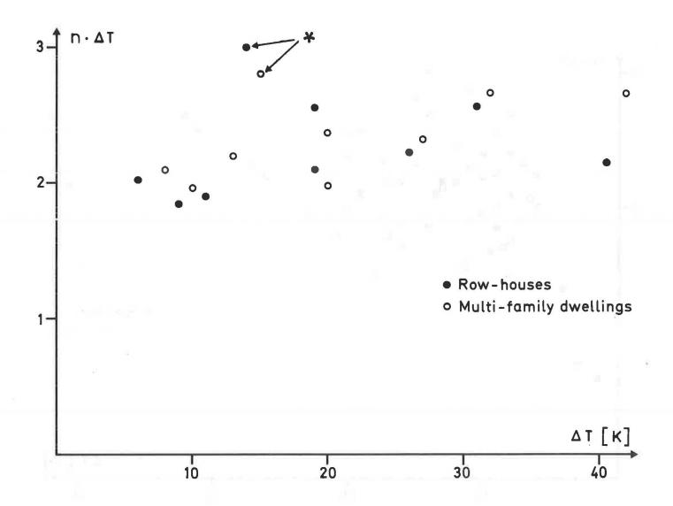
Fig 2 Fraction of rooms having open windows, n, times the indoor-outdoor temperature difference  $\Delta T$ , versus  $\Delta T$ . Data from observations of row-houses and multi-family buildings performed in this investigation. Data points indicated by an asterisk refer to days when there was someone at home in a large fraction of the households.
