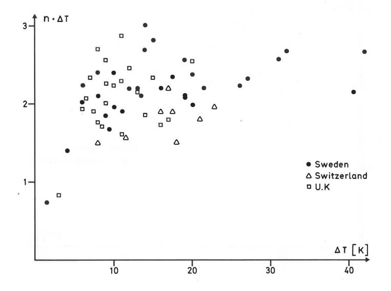
Fig 3 Fraction of rooms having open windows, n, times the indoor-outdoor temperature difference ΔT, versus ΔT. Data from eight studies (ref 4, 6, 7, 11 and this investigation) in Sweden, Switzerland and the UK.
