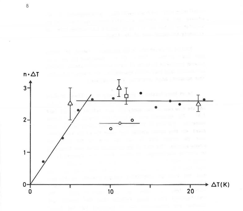
Fraction of rooms having open windows, n, times the indoor-outdoor temperature differences ΔT, versus ΔT. o pilot study of ref 7
