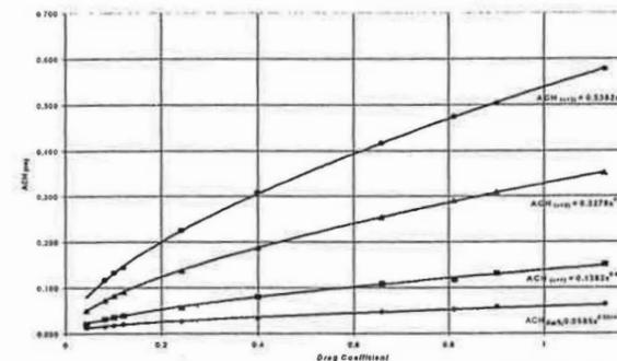
Figure 2b. Fitting curves of location-averaged winter ACH (closed windows) as a function of Cd, for various wind velocities.
