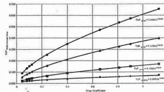
Figure 2a. Fitting curves of location-averaged TUF<sub>nv(H)</sub> as a function of Cd, for various wind velocities.
