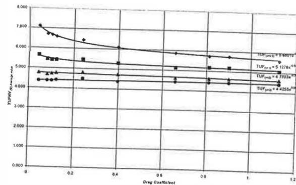
Figure 3a. Fitting curves of locations-averaged TUFnv(C) as a function of Cd, for various wind velocities.
