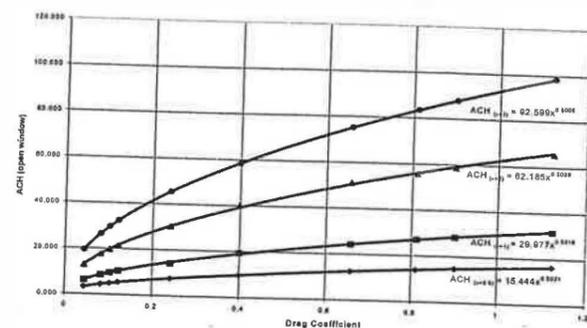
Figure 3b. Fitting curves of location-averaged summer ACH (open windows) as a function of Cd, for various wind velocities.
