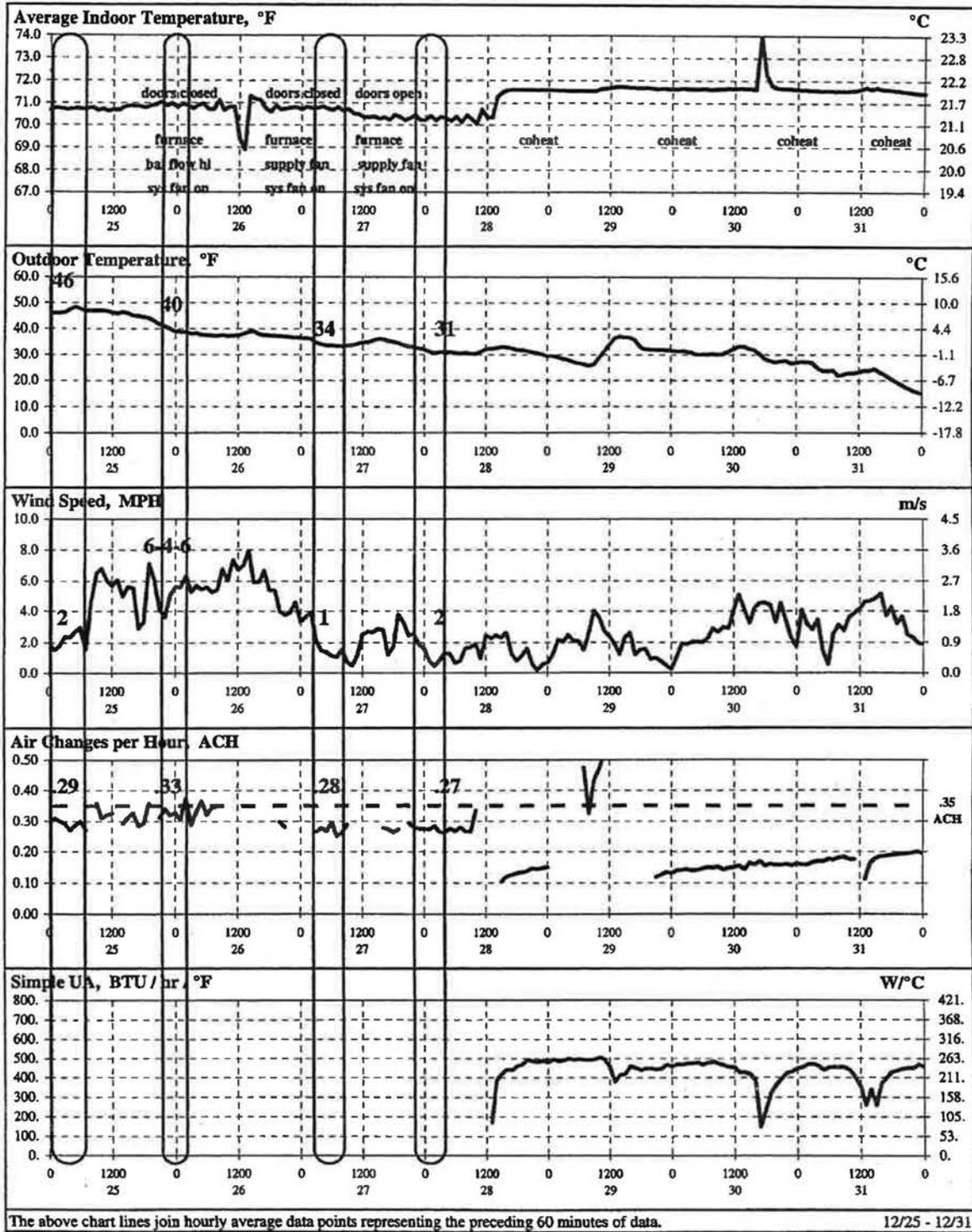
Figure 11 Short term energy monitoring (STEM) test and ventilation test data—lab house, Pittsburgh, Pa., December 25-31, 1997.
