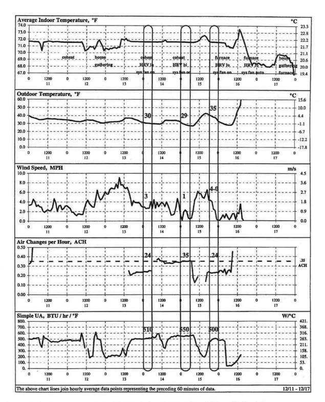
Figure 9 Short term energy monitoring (STEM) test and ventilation test data—lab house, Pittsburgh, Pa., December 11-17, 1997.
