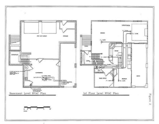
Figure 2 (Left) basement level HVAC plan, and (right) 1st floor level HVAC plan.
