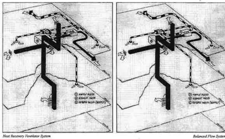
Figure 5 (Left) heat recovery ventilator system, and (right) balanced flow system.
