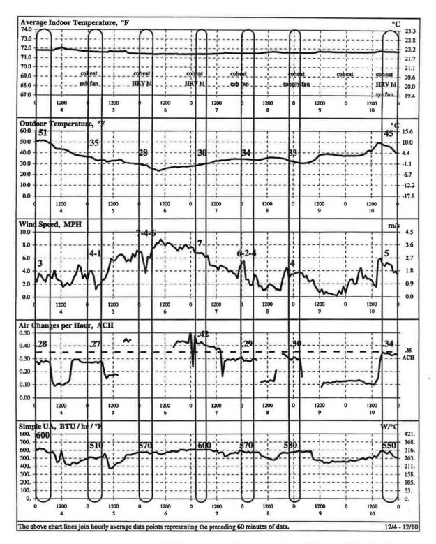
Figure 8 Short term energy monitoring (STEM) test and ventilation test data—lab house, Pittsburgh, Pa., December 4-10, 1997.
