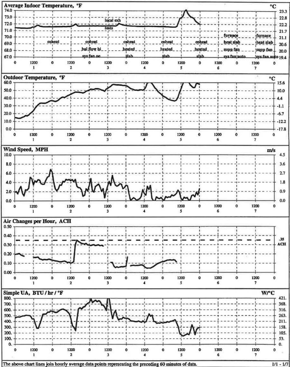
Figure 12 Short term energy monitoring (STEM) test and ventilation test data—lab house, Pittsburgh, Pa., January 1-7, 1998.
