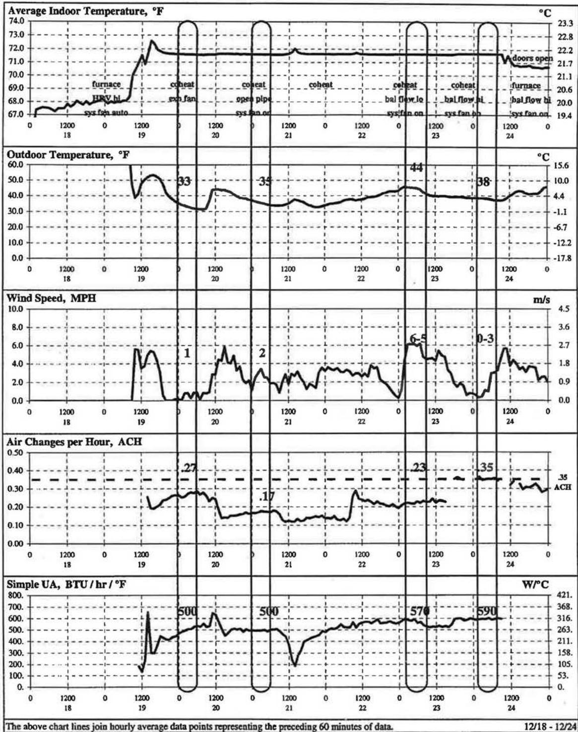
Figure 10 Short term energy monitoring (STEM) test and ventilation test data—lab house, Pittsburgh, Pa., December 18-24, 1997.
