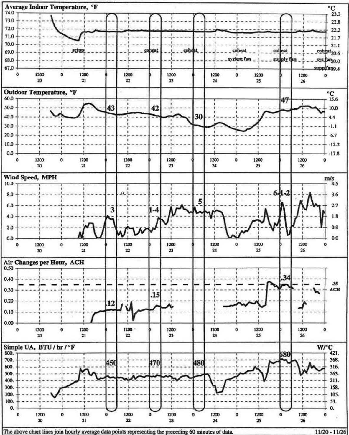
Figure 6 Short term energy monitoring (STEM) test and ventilation test data—lab house, Pittsburgh, Pa., November 20-26, 1997.
