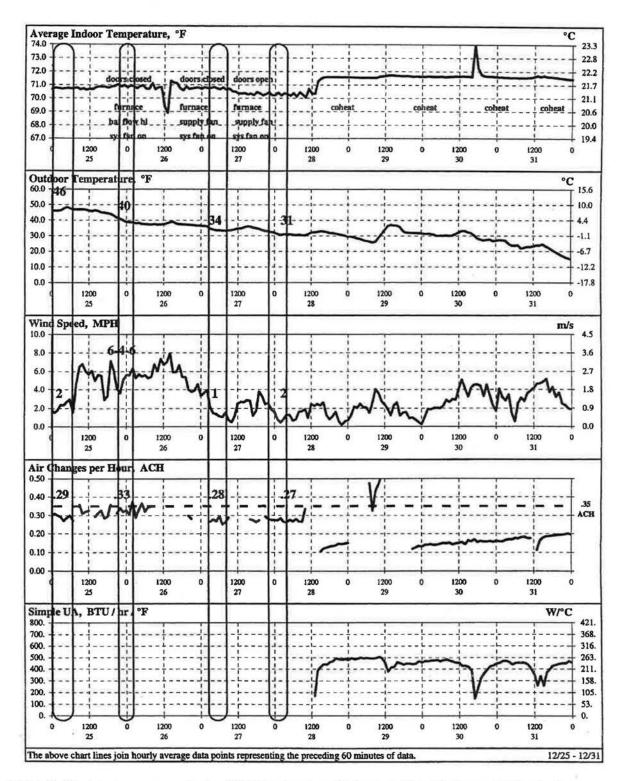
Figure 11 Short term energy monitoring (STEM) test and ventilation test data—lab house, Pittsburgh, Pa., December 25-31, 1997.
