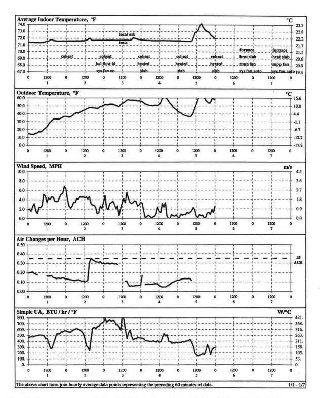
Figure 12 Short term energy monitoring (STEM) test and ventilation test data—lab house, Pittsburgh, Pa., January 1-7, 1998.
