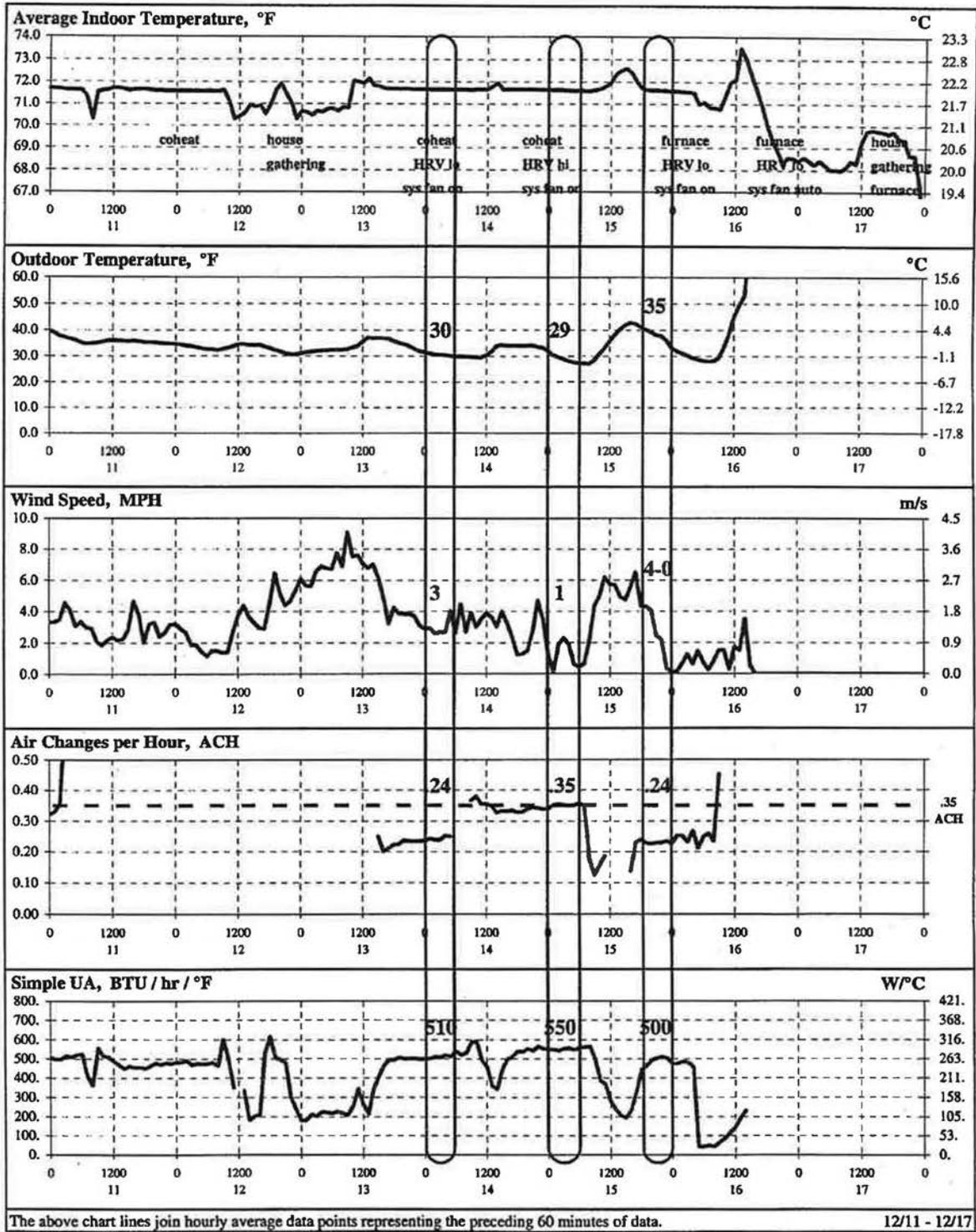
Figure 9 Short term energy monitoring (STEM) test and ventilation test data—lab house, Pittsburgh, Pa., December 11-17, 1997.
