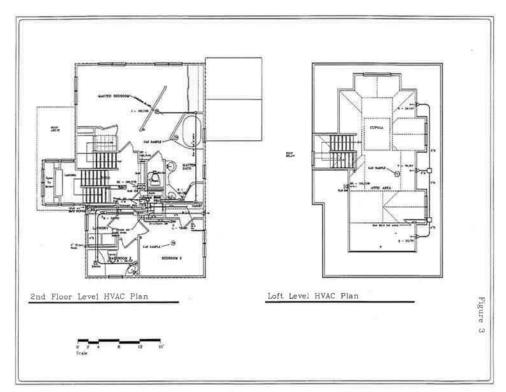
Figure 3 (Left) 2nd level HVAC plan, and (right) loft level HVAC plan.
