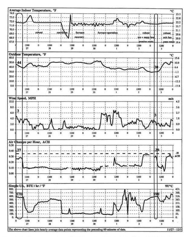
Figure 7 Short term energy monitoring (STEM) test and ventilation test data—lab house, Pittsburgh, Pa., November 27-December 3, 1997.
