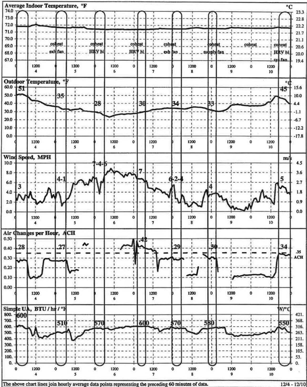
Figure 8 Short term energy monitoring (STEM) test and ventilation test data—lab house, Pittsburgh, Pa., December 4-10, 1997.
