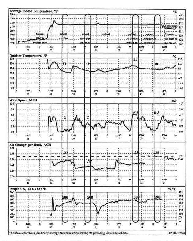
Figure 10 Short term energy monitoring (STEM) test and ventilation test data—lab house, Pittsburgh, Pa., December 18-24, 1997.
