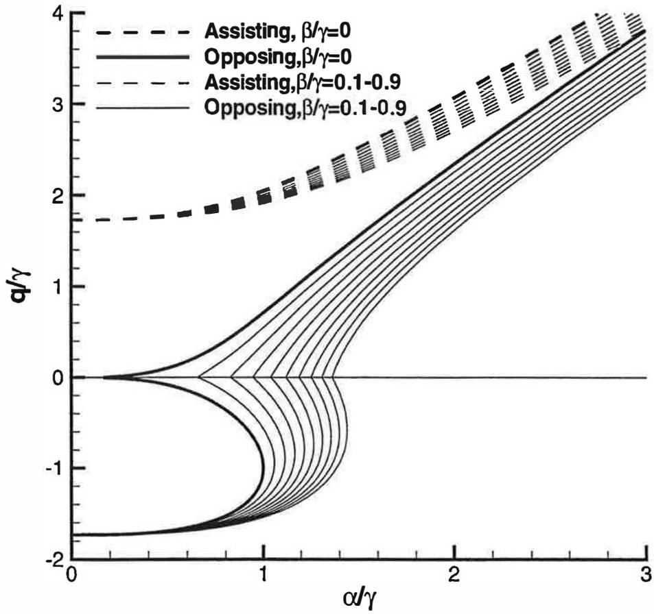
Figure 3. Scaled flow rate as a function of the scaled heat gain parameter  $\alpha_D$  and heat loss parameter  $\beta$  for both assisting and opposing winds. For opposing winds the parameters for the two zones have been chosen to give a solution behaviour corresponding to Fig. 2b.
