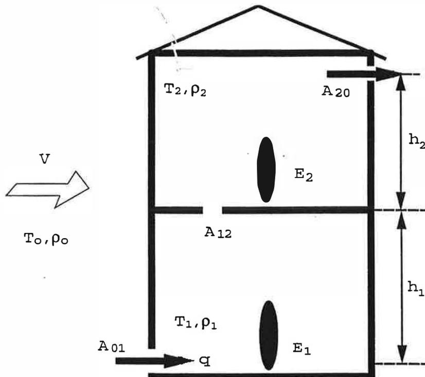
Figure 1. Geometry and notation for the two-zone building.
