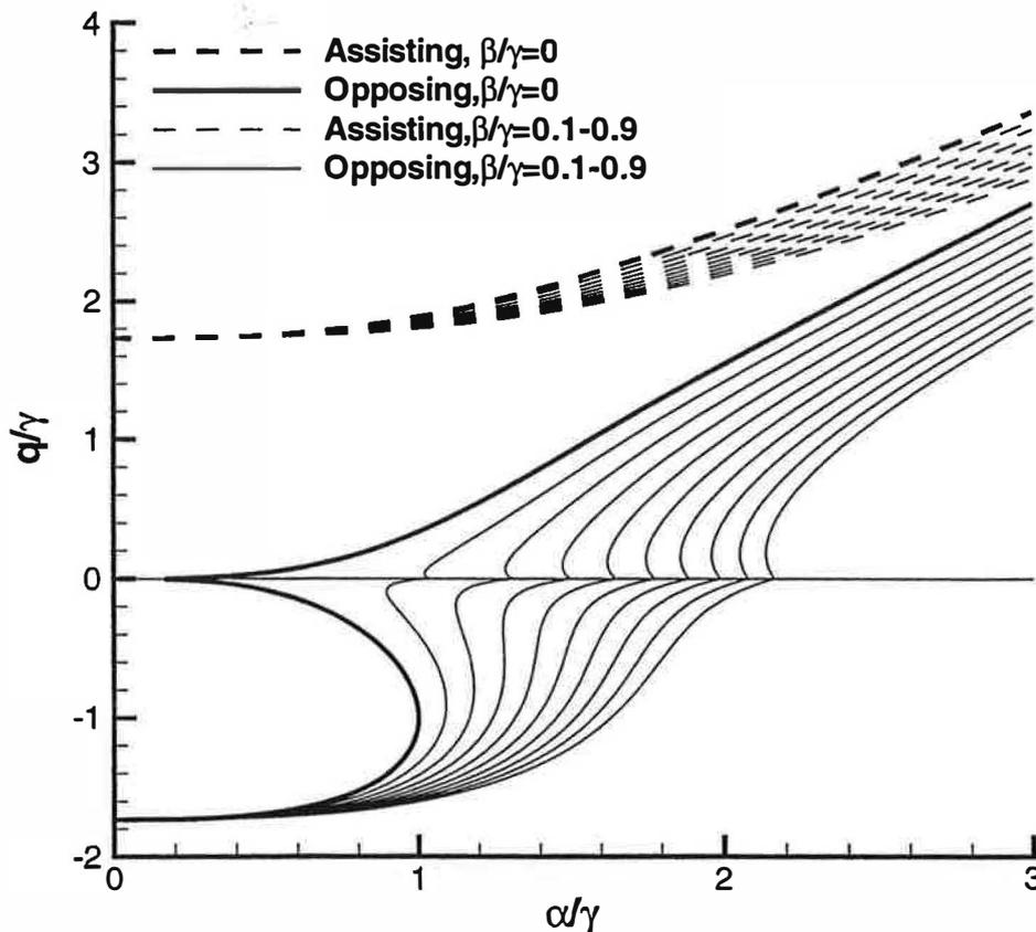
Figure 4. Scaled flow rate as a function of the scaled heat gain parameter  $\alpha_D$  and heat loss parameter  $\beta$  for both assisting and opposing winds. For opposing winds the parameters for the two zones have been chosen to give a solution behaviour corresponding to Fig. 2d (for small  $\beta/\gamma$ ) or Fig. 2c (for larger  $\beta/\gamma$ ).
