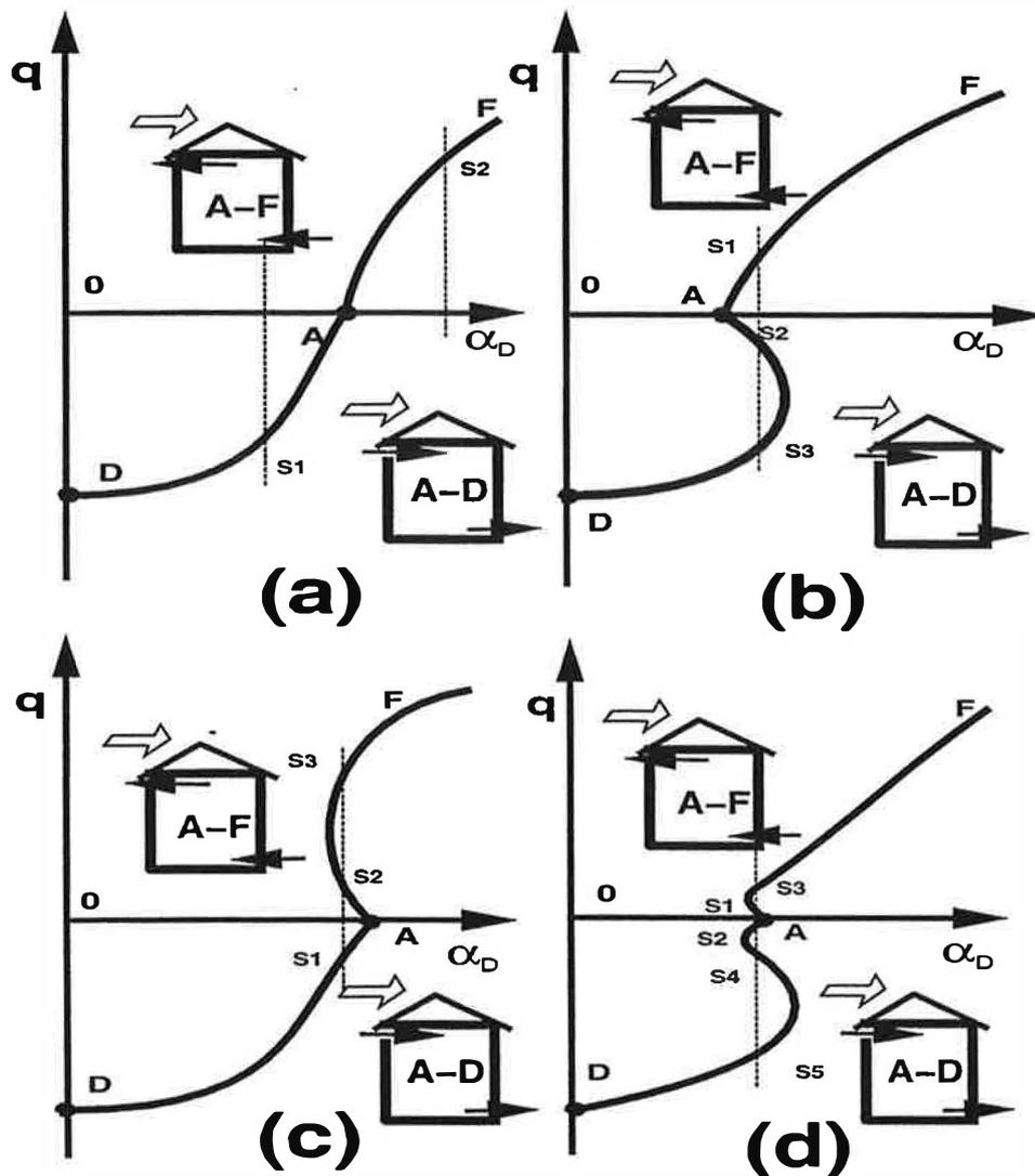
Figure 2. Some possible behaviours of the flow rate  $q$  for opposing winds as a function of the heat gain parameter  $\alpha_D$ . Positive  $q$  indicates upward flow; negative  $q$  indicates downward flow.
