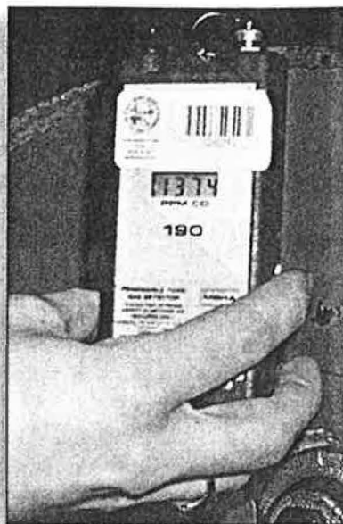
FIGURE 2. Carbon monoxide detector showing a high reading (1374 ppm) during a radon investigation at an unoccupied school. This incident is exemplary of the need to measure carbon monoxide levels routinely during IAQ investigations.
