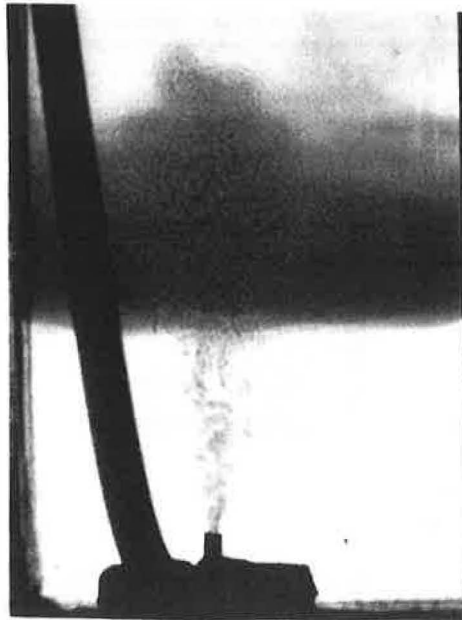
Figure 4b Photograph of exchange flow interacting with a plume of buoyant fluid released at the floor.
