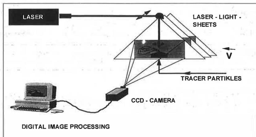
Figure 2 Principle of laser-light-sheet method with digital image processing
