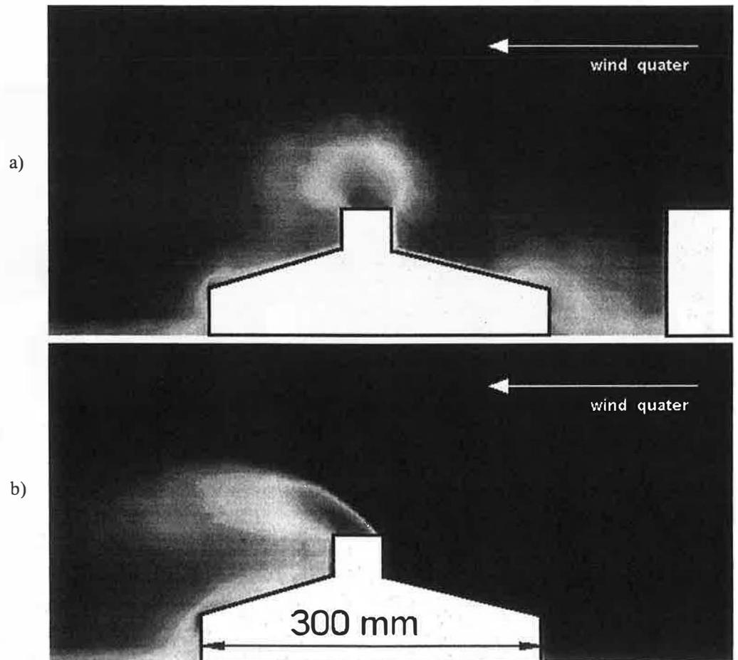
Figure 4 Laser-light-sheet frame (averaged frame, derived from 100 single frames) of a natural ventilated livestock building with single outlet
