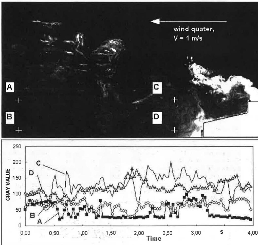
Figure 3 Fluctuation of gray values at points A, B, C and D at the lee region of a cross ventilated livestock building with natural ventilation
