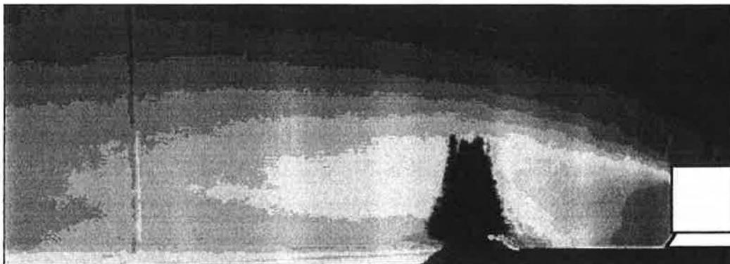
Figure 6 Same conditions as described for figure 5, additional barriers upwind and downwind with vegetative windbreaks planted on top of them
