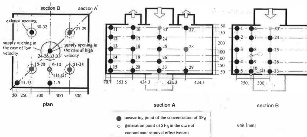
Figure 2 Measuring point and generation point of SF<sub>6</sub>
