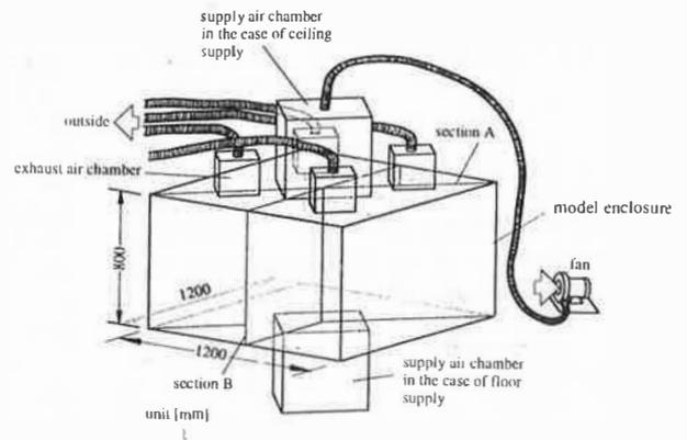
Figure 1 Model of the room mechanically ventilated
