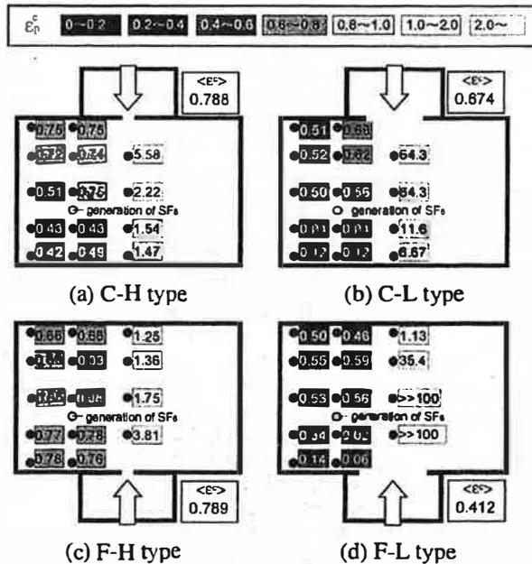
Figure 5 Distribution of local air quality index (section B, the generation point of  $SF_6$ : (1))
