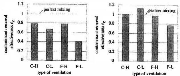
(a) SF<sub>6</sub> generation from point (1) (b) SF<sub>6</sub> generation from point (2)
