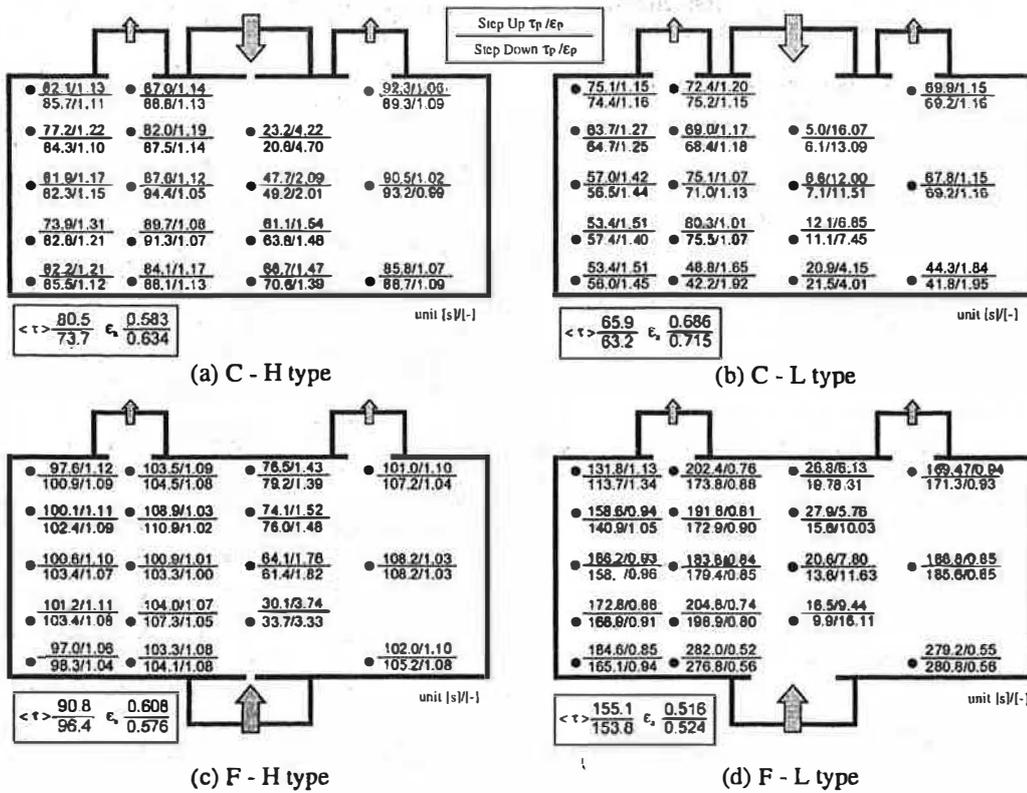
Figure 4 Distribution of local mean age of air and local air change index (section A)
