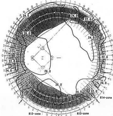
Figure 4 Temperature distribution (°C) in Case 1 (basic condition)
