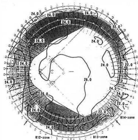
Figure 6 Temperature distribution (°C) in Case 3 (circulating airflow fans : on)
