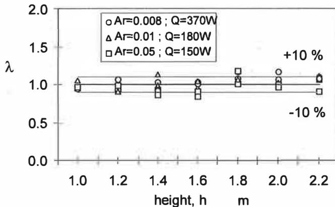
Fig. 5 The temperature and velocity profiles widths ratio  $\lambda$ , versus height above the heat source.
