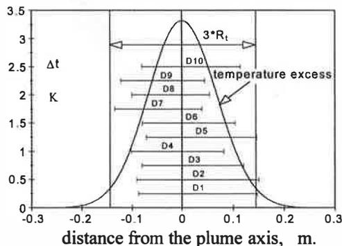
Fig. 3 Comparison of temperature excess distributions in a buoyant plume and the plume diameter observed during flow visualisation
