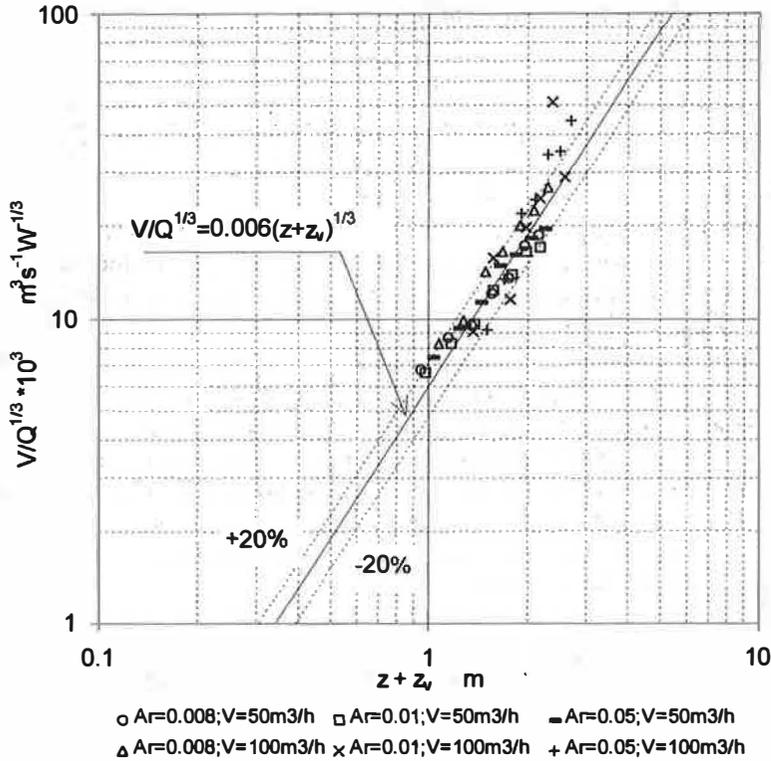
Fig. 6 Air volume flux increase in buoyant plumes with displacement ventilation
