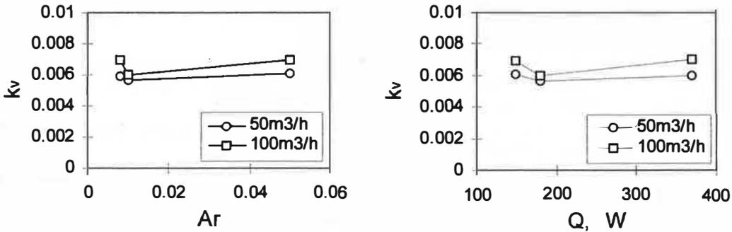
Fig. 7 Coefficient  $k_v$  dependence on  $Ar_0$  and  $Q_0$
