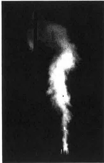
Figure 1. Smoke test with convective heat source (900 W)
