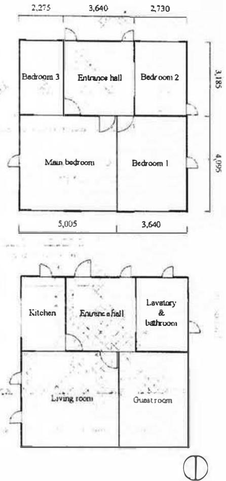
Figure 11. House plan for calculation of heating load
