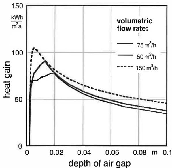
Figure 6: Heat gains of a facade system with translucent curtain wall specific to the solar aperture area for heating period (October to April)
