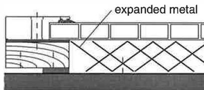
Figure 4: Facade detail with expanded metal
