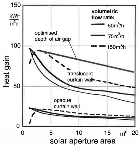
Figure 7: Heat gains of systems with translucent or opaque curtain wall for different volumetric flow rates specific to solar aperture area for heating period
