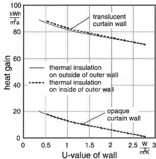
Figure 5: Heat gains of a facade system with translucent or opaque curtain wall mounted on backing wall of varying U-value (in comparison to insulated standard wall) specific to the solar aperture area for heating period (October to April)
