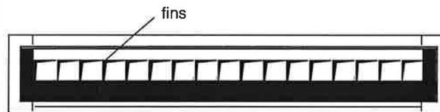
Figure 3: Cross section through a commercial air collector with fins (type: "Grammer" [5])
