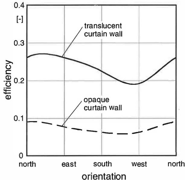
Figure 8: Efficiency of systems with translucent or opaque curtain wall for different orientations
