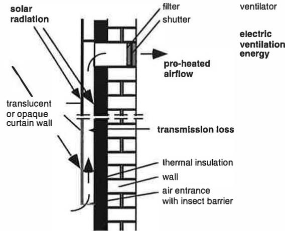
Figure 1: Function principle of the system
