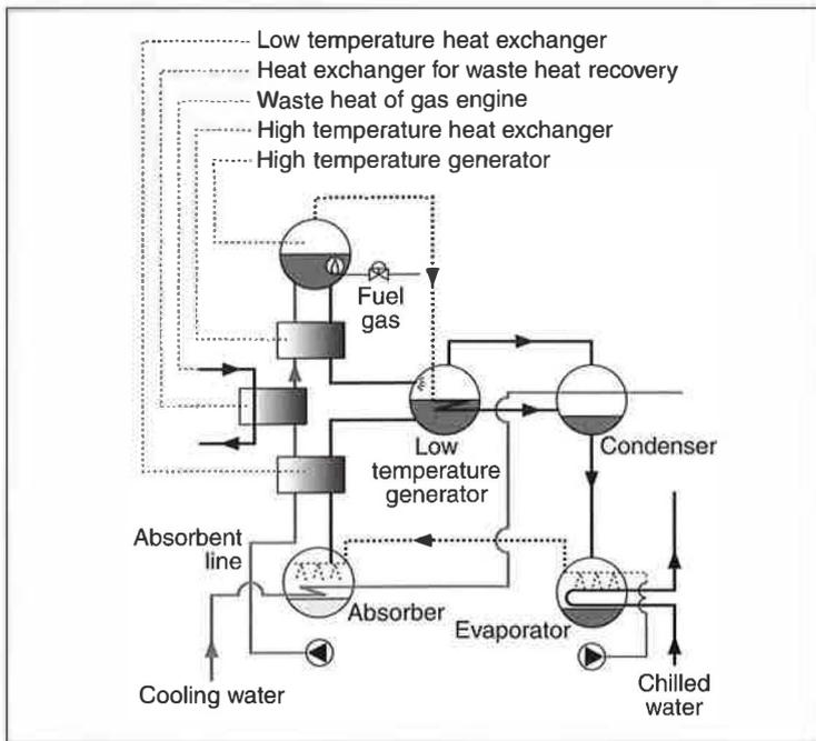
Figure 2: Flow diagram of the waste-heat input absorption chiller-heater.
