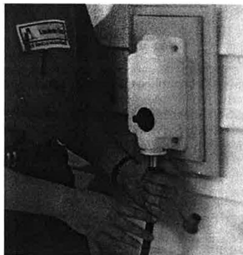
Figure 5 — The Gas Convenience Outlet, from M.B. Sturgis (Maryland Heights, Missouri), makes it safe and easy to connect and disconnect gas ranges, clothes dryers, outdoor grills, etc. Manual on-off and automatic shut-off valves with a safety interlock prevent connection or disconnection of an appliance when the outlet is in the "on" position. Built-in thermal protection prevents gas flow if the outlet is exposed to temperatures in excess of 200°F.
