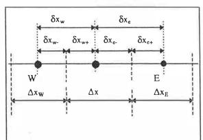
Figure 3 Grid points for x direction
