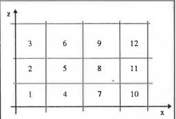
Figure 4 Two dimensional grid and the order of elements in the state vector
