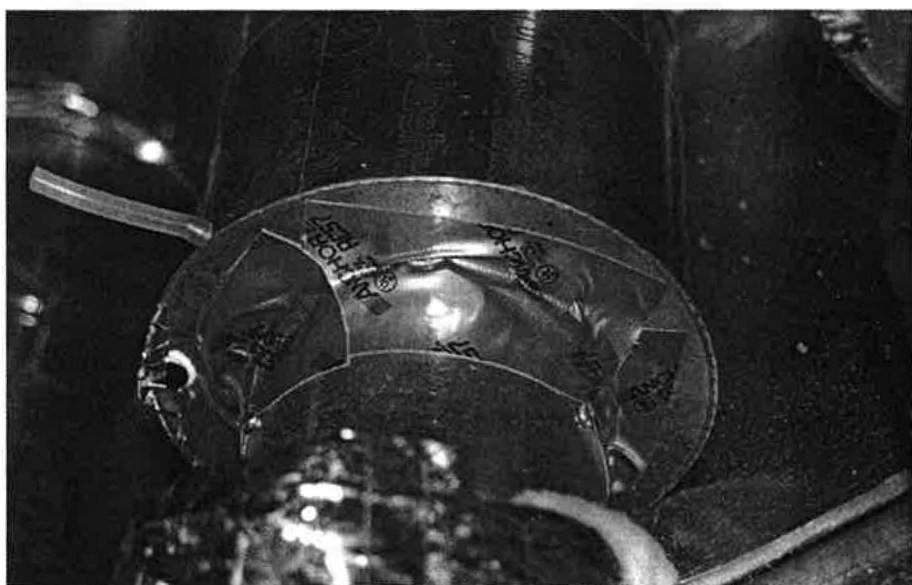
Duct tape can form a good seal—initially. But under the challenging conditions of the aging rig, it quickly fails.
