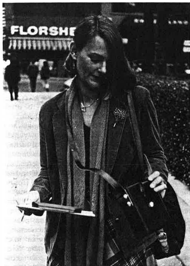
Fig. 1. Method of taking a CO measurement in downtown San Francisco using General Electric personal exposure monitor.
