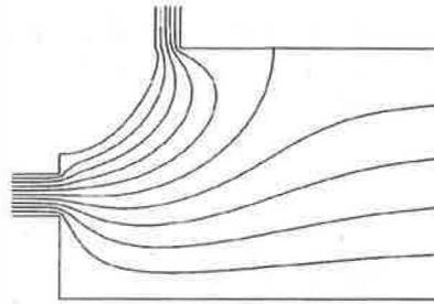
Figure 6: Potential fluid flow streamlines in the geometrical model, see figure 3, using the mapped ellipse method, with the sash of strength  $0.25 m^2 s^{-1}$  and the ventilation duct of strength  $0.125 m^2 s^{-1}$ . The values of the stream function along each streamline are from  $-0.225$  to  $-0.025$  in steps of  $0.025$ .
