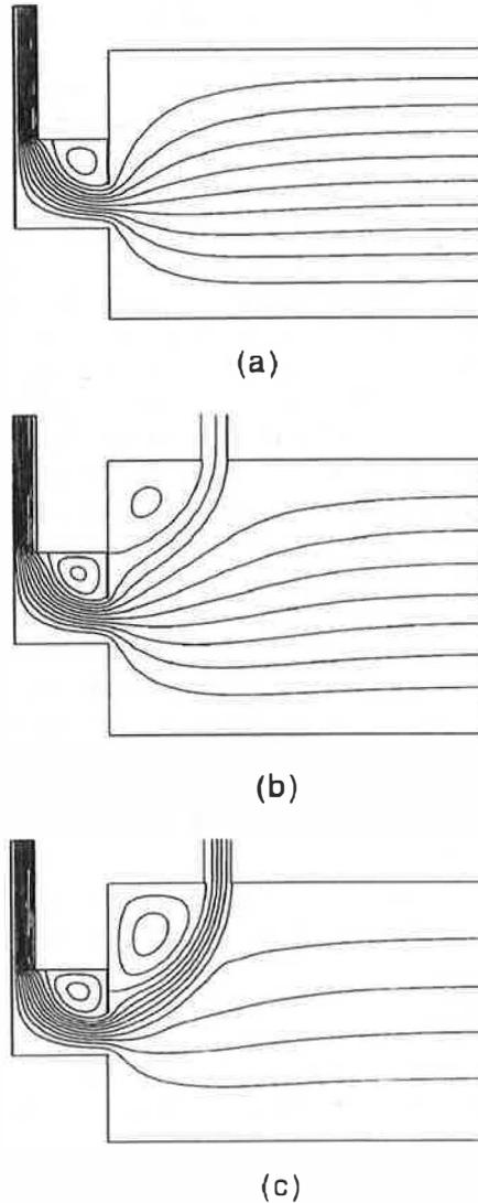
Figure 2: Turbulent fluid flow streamlines in the physical region, see figure 1, with the flux of the fluid through exhaust duct being  $0.25 \text{ m}^2 \text{ s}^{-1}$  and the flux of the fluid through the ventilation duct being (a)  $0 \text{ m}^2 \text{ s}^{-1}$ , (b)  $0.05 \text{ m}^2 \text{ s}^{-1}$ , and (c)  $0.125 \text{ m}^2 \text{ s}^{-1}$ . The values of the stream function along each streamline are from  $-0.3$  to  $-0.025$  in steps of  $0.025$ .
