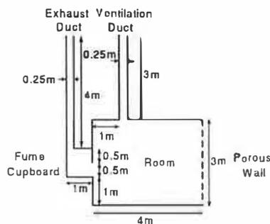
Figure 1: Physical dimensions of the room, fume cupboard and ventilation duct.
