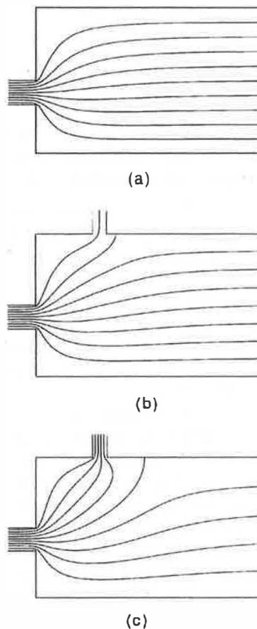
Figure 4: Potential fluid flow streamlines in the geometrical model, see figure 3, with the sash of strength  $0.25 \text{ m}^2 \text{ s}^{-1}$  and the ventilation duct of strength (a)  $0 \text{ m}^2 \text{ s}^{-1}$ , (b)  $0.05 \text{ m}^2 \text{ s}^{-1}$ , and (c)  $0.125 \text{ m}^2 \text{ s}^{-1}$ . The values of the stream function along each streamline are from  $-0.225$  to  $-0.025$  in steps of  $0.025$ .
