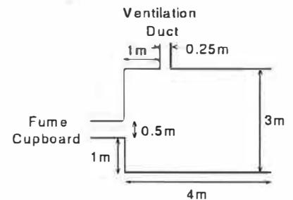
Figure 3: Simplified geometrical model.
