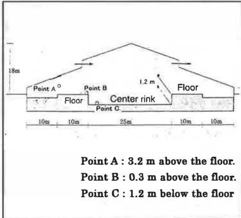
Figure.2 Main measuring points
