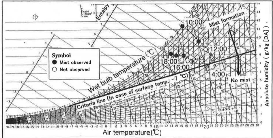
**Figure. 5 Criteria line for preventing mist formation and measurement results at an indoor skating rink**
